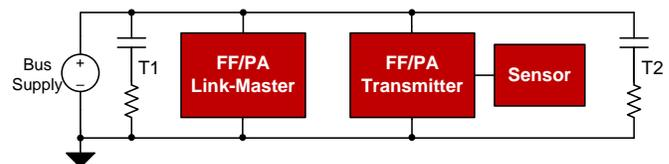
Figure 1. FF/PA Fieldbus Network
