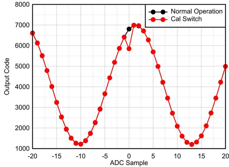
Figure 3-3. ADC32RF55 Output Codes During Foreground Calibration
