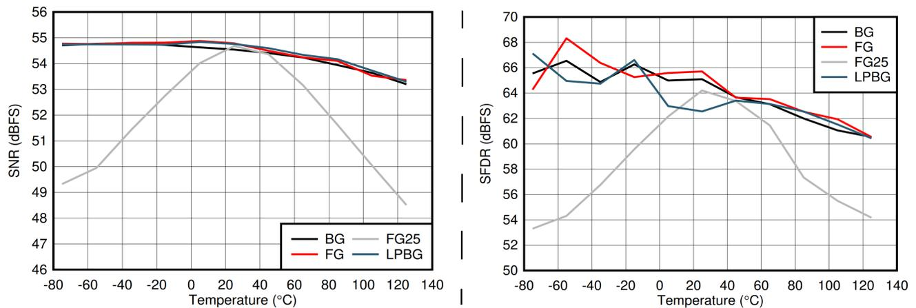
**Figure 2-1. ADC12DJ5200RF Performance Versus Temperature in Different Calibration Modes**
