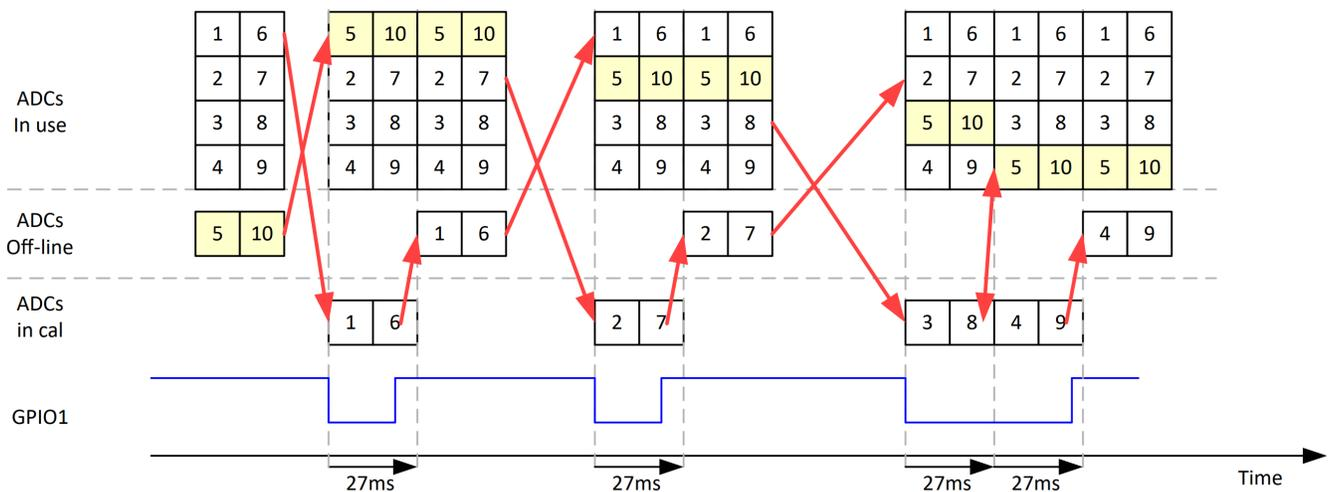
Figure 3-4. ADC32RF55 Core Swap During Background Calibration
