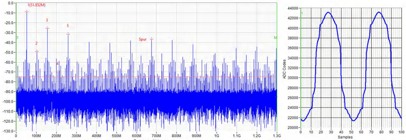
**Figure 3-1. ADC32RF55 Output Without One-time Calibration**
