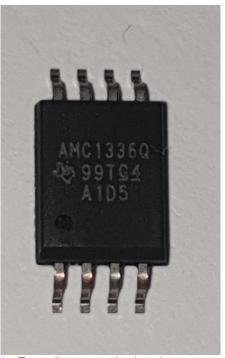
Figure 1 Device under Test, all test samples has the same package size
