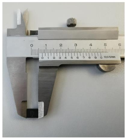
Figure 2 Measuring of Clearance and Creepage
