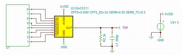
Figure 1. Parallel Precision DAC Model in TINA-TI Schematic
