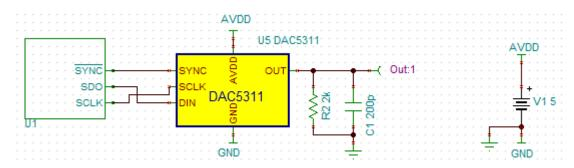
Figure 2. Serial Precision DAC Model in TINA-TI Schematic
