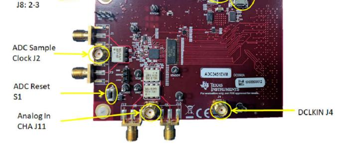
Figure 2-1. ADC354xEVM Feature Identification
