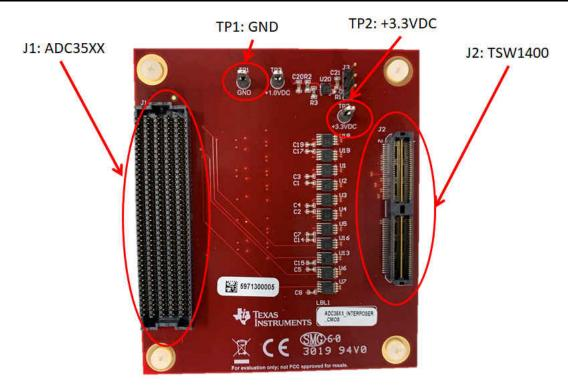
Figure 2-2. CMOS FPGA Interposer
