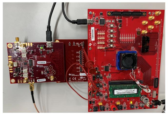
Figure 3-1. ADC3660EVM Full Setup
