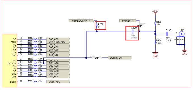
Figure 5-1. ADC3660EVM Schematic Snippet: DCKLIN
