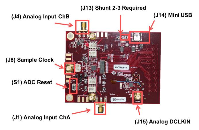
Figure 2-1. ADC3660EVM Feature Identification
