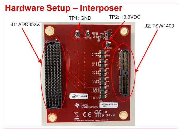
Figure 2-2. CMOS FPGA Interposer Card
