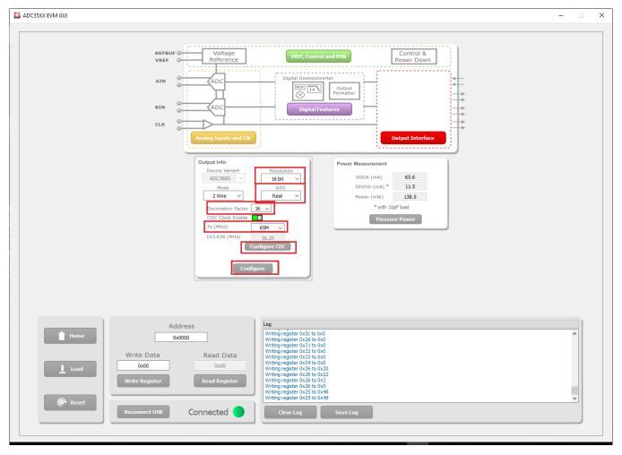
Figure 4-8. ADC35xx GUI settings for Real Decimation Mode
