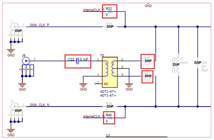
Figure 5-2. ADC3660EVM Schematic Snippet: Sample Clock
