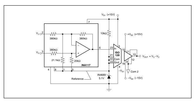
FIGURE 6. Single Supply Isolation Amplifier with High Common-Mode Range Differential Inputs.
