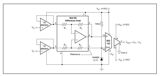
FIGURE 4. Single Supply (almost-see text), Isolation Amplifier with High-Impedance Differential Inputs..
