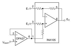
Figure 1. Level Shifting Circuit Using the INA105's  $V_{\mbox{\tiny REF}}$  Pin
