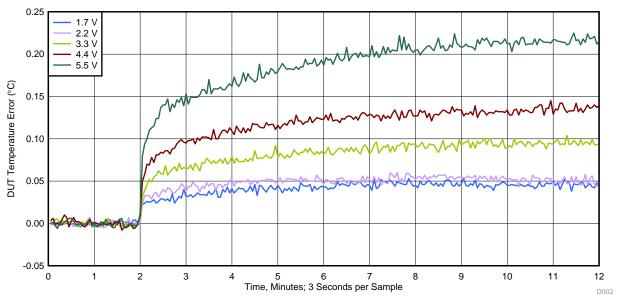
On second minute, TMP107 is switched from one shot mode to continuous 15-ms conversion mode. Data is read back every 3 s.
