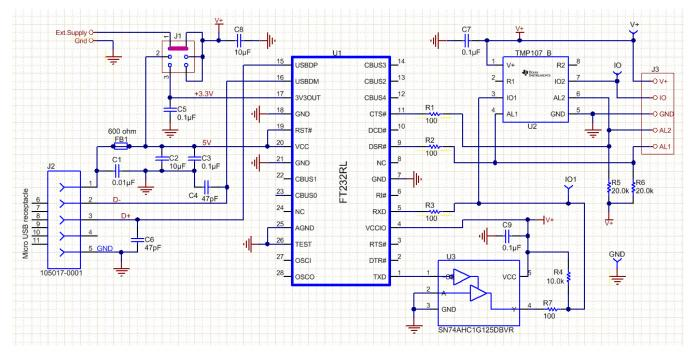
Figure 6. Example USB Port-Based Control Board
