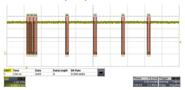
Figure 11. Oscilloscope of 4 Parts Chain Initialization Signal
