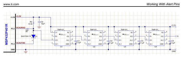
Figure 7. Example Microcontroller-Based Control Board
