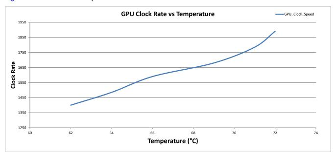
Figure 4-5. Gaming PC: GPU Clock Rate vs Temperature
