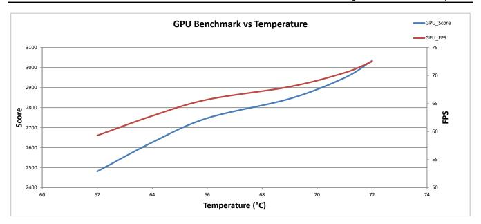
Figure 4-7. Gaming PC: GPU Benchmark Score vs Temperature
