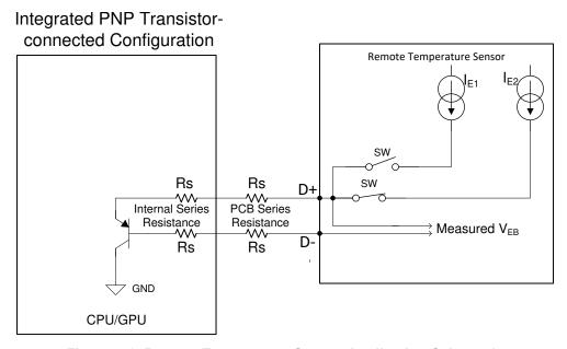
Figure 5-2. Remote Temperature Sensor Application Schematic
