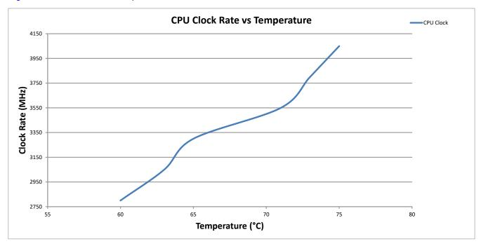
Figure 4-2. Gaming PC: CPU Clock Rate vs Temperature
