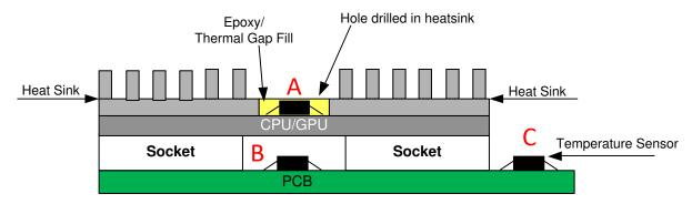
Figure 5-1. Local Temperature Sensor Placements
