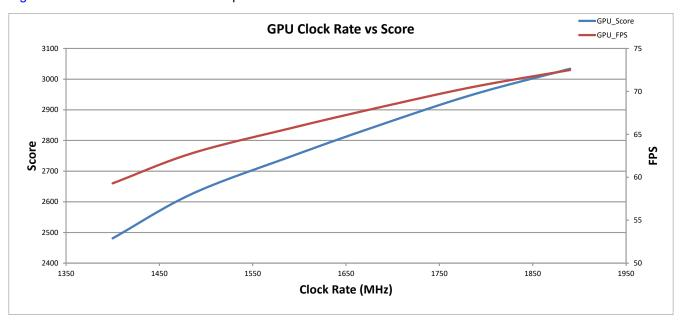
Figure 4-6. Gaming PC: GPU Benchmark Score vs Clock Rate
