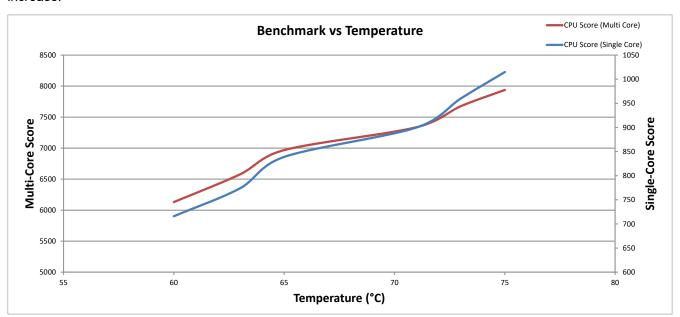
Figure 4-4. Gaming PC: CPU Benchmark vs Temperature
