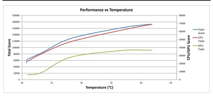
Figure 4-1. Smartphone: Benchmark Scores vs Temperature
