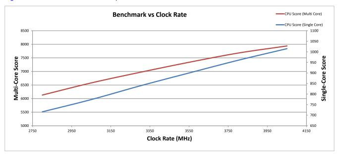
Figure 4-3. Gaming PC: CPU Benchmark vs Clock Rates
