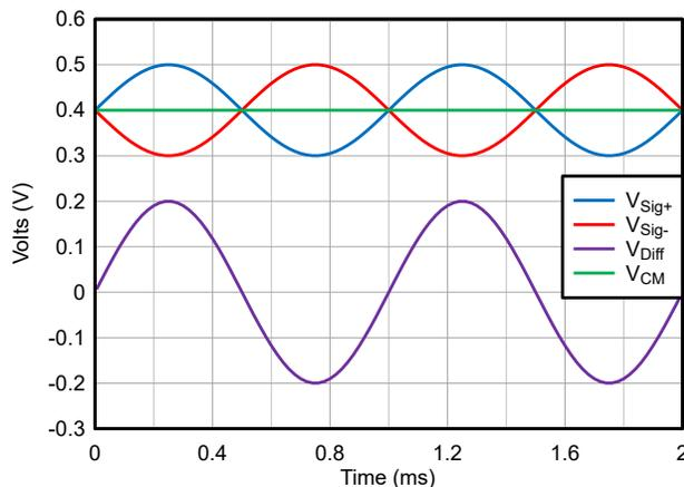
**Figure 1-1. AC Differential Signal with DC Common-Mode Voltage**
