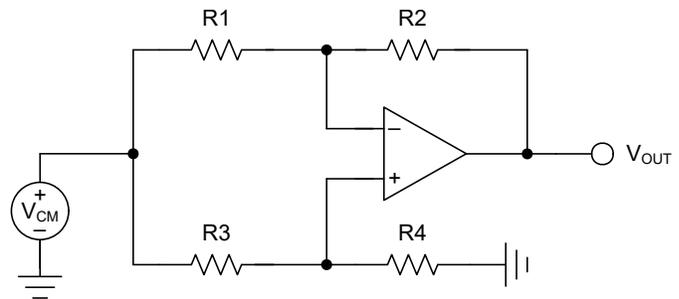
**Figure 4-4. Superposition: Common-Mode**
