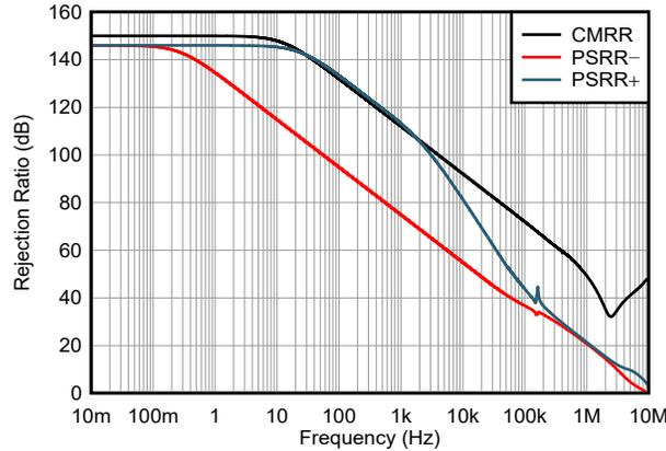
**Figure 2-2. PSRR and CMRR vs Frequency, OPA387**
