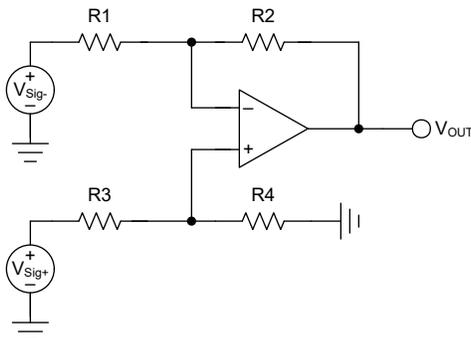
**Figure 2-1. Difference Amplifier Circuit**
