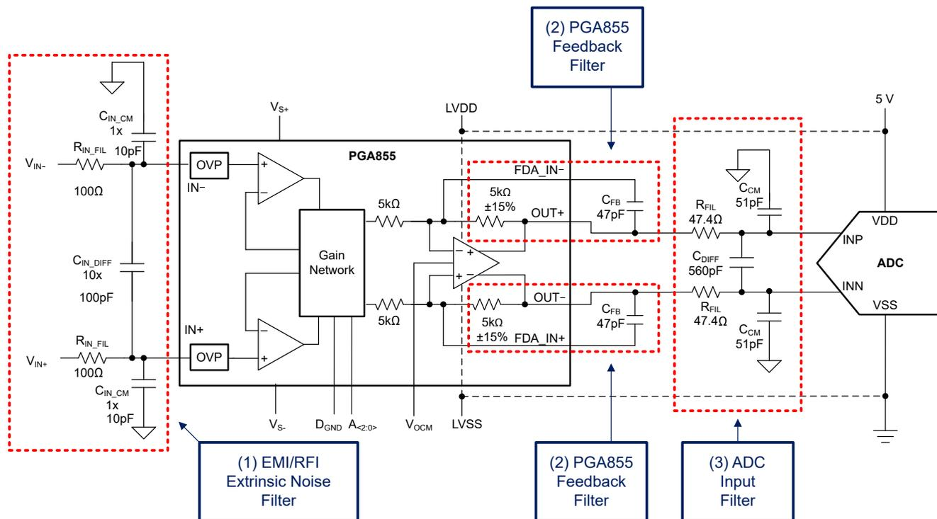
Figure 2-1. PGA855 Analog Filters
