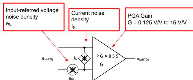
Figure 4-2. Simplified Noise Model for PGA855
