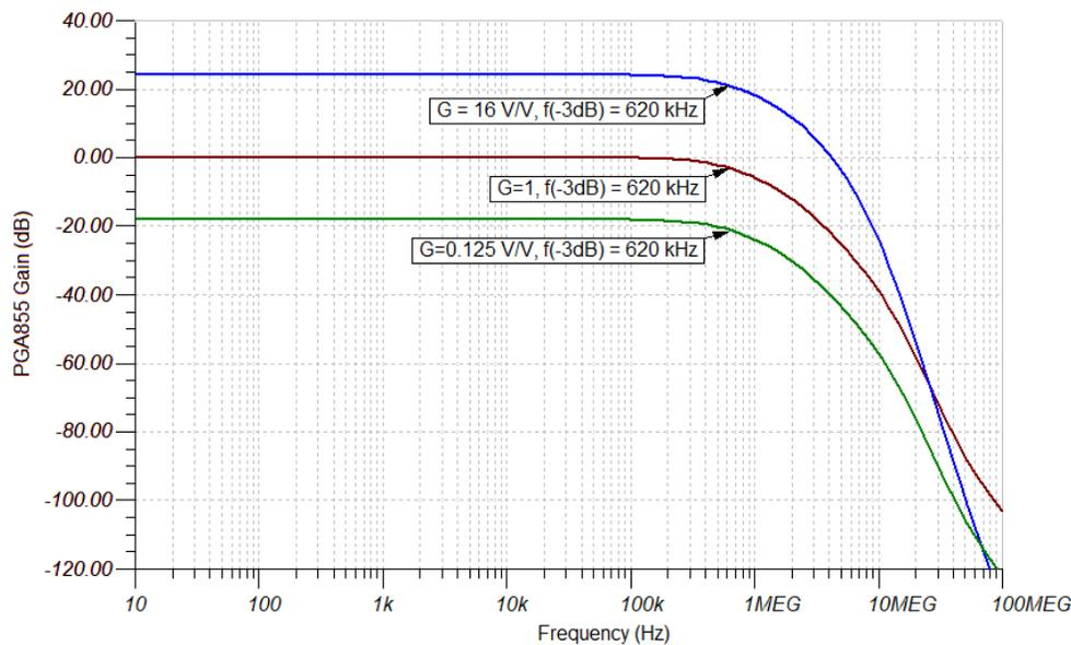
**Figure 2-2. PGA855 Frequency Response Simulation Result**
