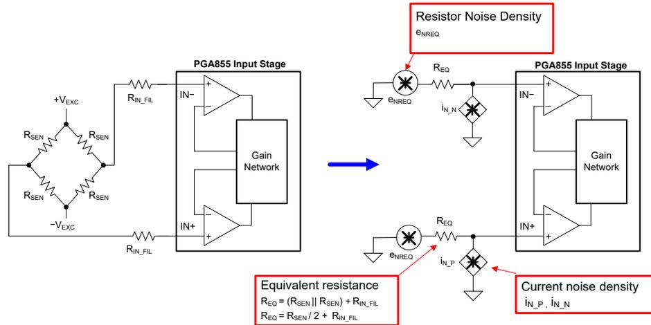
**Figure 4-4. PGA855 Current Noise and Source Resistance**
