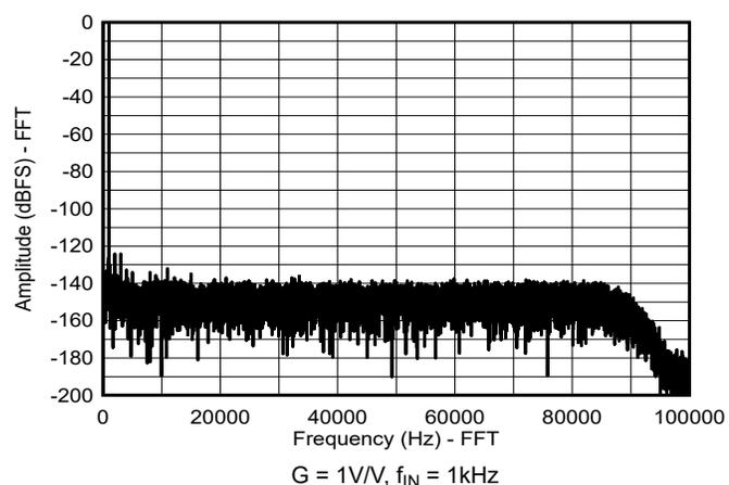
**Figure 7-2. Wideband Filter Performance**
