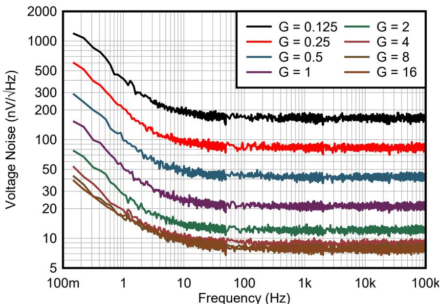
Figure 4-3. Voltage Noise Spectral Density of PGA855
