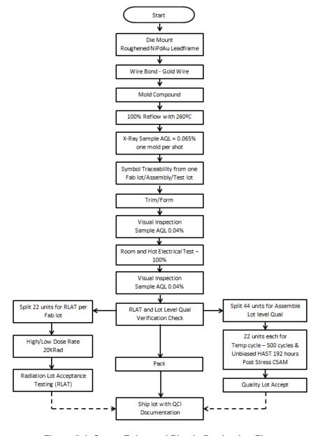
Figure 2-1. Space Enhanced Plastic Production Flow
