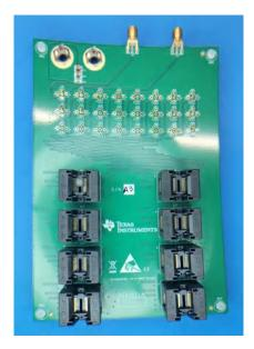
Figure 3-3. SN54SC4T125-SEP Evaluation Board (Top View)
