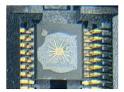
Figure 3-2. Photo of SN54SC4T125-SEP Package Decapped
