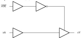
Figure 2-1. Functional Block Diagram of the SN54SC4T125-SEP
