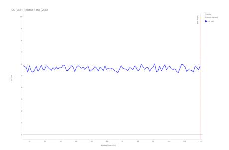
Figure 5-3. Current versus Time for Run 7 of the SN54SC4T125-SEP at T = 125°C
