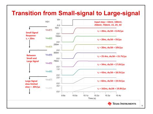
This figure illustrates the output of the non-inverting buffer circuit from the previous slide, versus different input step sizes.
