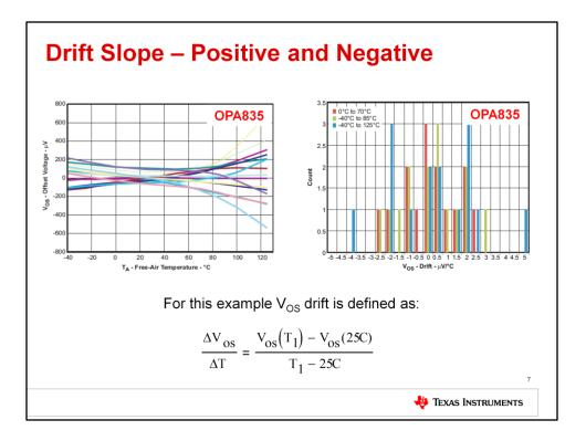
The slope on offset voltage drift can be either positive or negative. This formula shows one possible definition for offset drift. This formula will produce a positive or negative drift depending on the slope of the curve. Some other definitions use the absolute value, so you will not have a negative offset.
