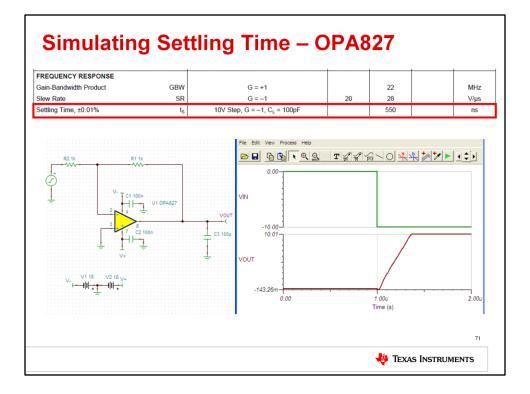
We can very easily simulate the settling time of an op-amp using TINA-TI's transient analysis function. In order to do this, it is important to closely follow the data sheet test conditions, such as the step size, gain configuration, and load capacitance.
