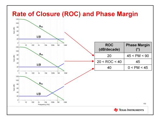
As shown in the previous slides, rate of closure and phase margin are closely connected. We can predict one value based on the other, and this slide gives three different examples of rate of closure and their corresponding phase margins.
