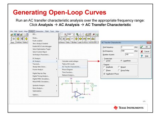
Once you've verified the DC functionality of the circuit, perform an AC transfer characteristic analysis over the op-amp bandwidth. Click Analysis, AC Analysis, AC Transfer Characteristic to do this.
