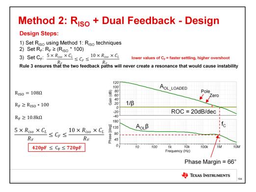
The first design step in this circuit is to select Riso. The same method that was used to select Riso in "Method 1: Riso" is used here, and Riso is selected to produce a zero in the Aol curve at f(Aol = 20dB).
