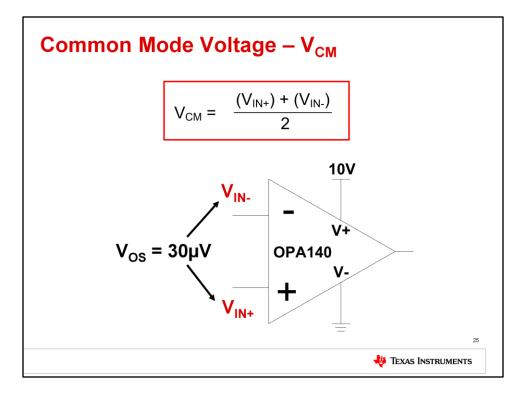
Common mode voltage is defined as the average voltage which is applied to the two inputs of an amplifier. In the case of an op amp, the two inputs are at the practically same potential, with only a small offset between them. So, effectively you can see the common mode voltage on either input.
