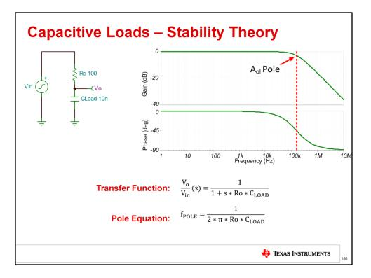
The AC transfer function of the equivalent load RC circuit has been plotted here. The pole location can be calculated from the transfer function and is shown at the bottom of the slide.
