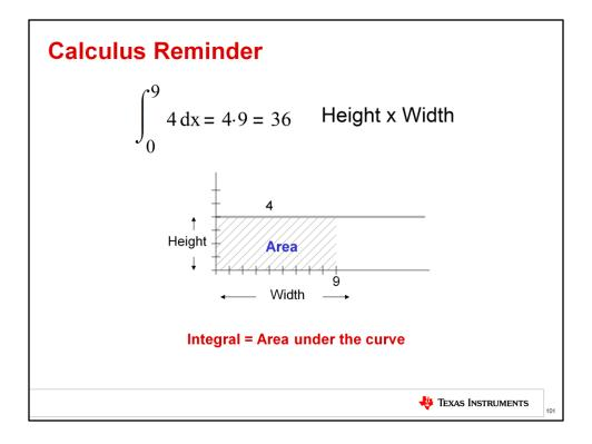
In order to gain a deeper understanding of the conversion from spectral density to RMS, we will need to use a little calculus. As a quick reminder, remember that the integral of a function is the area under its curve. The area of a rectangle is simply the width times the height, so the integral of a rectangle is also the width times the height. This simple fact will be useful in doing a dimensional analysis for noise.
