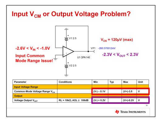
Lets look at another example. Note that this circuit has a different power supply arrangement, where the supplies are +/-2.5V.
