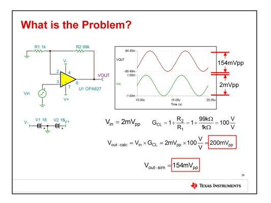
In this transient simulation, the OPA827 is set up in a non-inverting configuration with a closed loop gain of 100V/V. The input signal, Vin, is 2mVpp. The product of the input signal and closed loop gain is 200mVpp.
