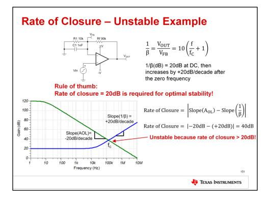
This method is called rate of closure analysis. To use this method, we only need to consider the gain plots of AoI and 1/B. These plots have well-defined slopes due to the poles and zeros in their transfer functions. By analyzing the rate of closure of AoI and 1/B at fC, the point where they intersect, we can quickly determine the stability of a circuit. The rule of thumb for this method is that the rate of closure at fc must equal 20dB for optimal stability.
