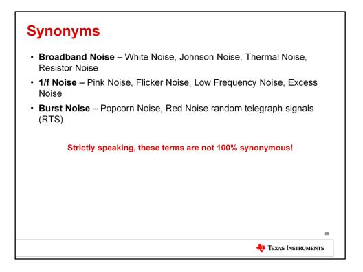
As we have already seen, the various categories of noise have many synonyms. For example, broadband noise is also called white noise, Johnson noise, thermal noise, and resistor noise. It can become very confusing to engineers that are new to this subject when literature and presentations switch between these different terms.
