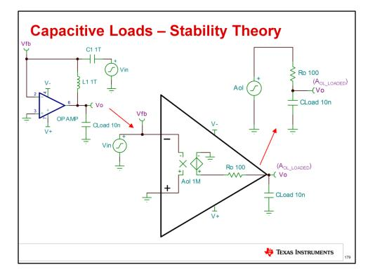
If we take a look at a simplified representation of the open-loop circuit, we see that the input signal passes through the Aol gain block and then the series open-loop output impedance, Ro, before reaching the op amp output, Vo. With a capacitor, Cload, on Vo, the op amp loaded Aol curve is divided down by an RC voltage divider.
