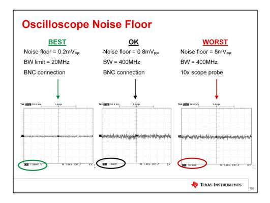
This slide shows a typical digitizing oscilloscope, measuring its noise floor in three different configurations. The worst configuration, shown on the right, has a noise floor of 8mVpp. In this case, a 10x scope probe is used and the scope bandwidth is set to the full 400MHz.
