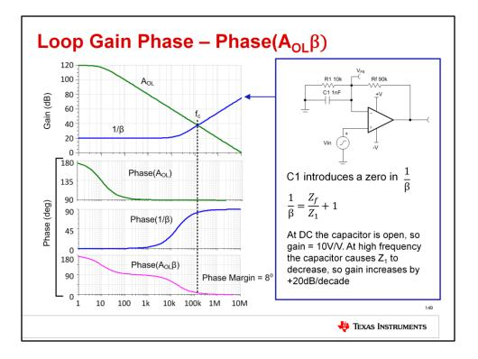
To measure the phase margin, we need to know the loop gain phase, or phase of AoIB, over frequency. Using the same log properties as before, we can simply subtract the phase of 1/B from the phase of AoI to get the phase of AoIB.
