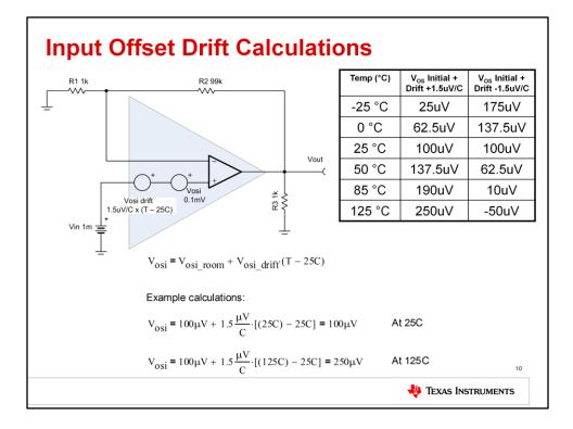
Offset drift calculations can be done in a similar manner. Notice that we have two sources: one for the initial offset and one for the offset drift. The offset drift source will be zero at 25C. As the temperature deviates from 25C, the temperature difference will be multiplied by the offset drift to generate the additional offset voltage.
