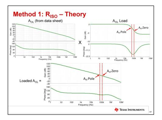
Adding the Aol and Aol load curves together as before, we can again see that the zero added by Riso cancels the pole in the Aol curve and restores the phase margin to an acceptable level for stability.
