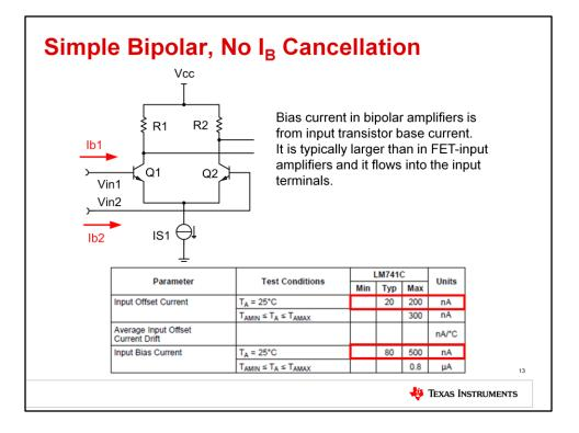
In a bipolar amplifier, input bias current is the current flowing into the base of each transistor in the input pair. Generally, the bias current for bipolar amplifiers is larger than the bias current for MOSFET and JFET amplifiers. Typical numbers are in the nA range. You can see in the case of the LM741C, the input offset current is about 200nA max, and the input bias current is about 500nA max.
