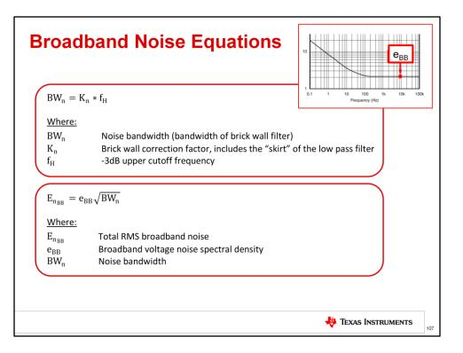
Now that we have the noise bandwidth relationship, we can use it to convert the op amp noise spectral density curve to RMS noise. The first equation given in this slide is the noise bandwidth equation that we have already discussed. Simply use the table on the previous slide to select the appropriate value for  $K_n$  and convert your signal bandwidth to noise bandwidth.
