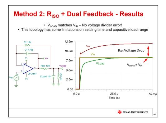
The results show that the output and load voltage arrive at the final level without excessive overshoot or ringing, indicating a stable system. The increase in Vo to overcome the voltage drop from Riso can also be clearly seen here.
