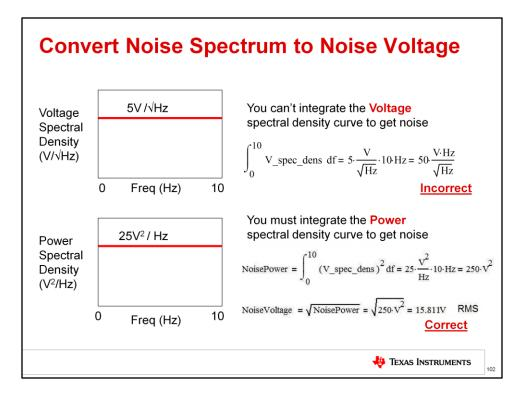
In this slide we will reiterate the method for converting from voltage spectral density to RMS voltage. A common misunderstanding with noise analysis is that total noise can be computed by integrating the **voltage** or **current** spectral density, when in fact you must integrate the **power** spectral density.
