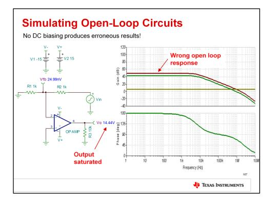
However, a circuit without feedback will not simulate properly because the output will go to one rail or the other. This causes incorrect Aol or output characteristics to be displayed. As shown here, the op-amp output is near the positive rail, resulting in an erroneously Aol curve.
