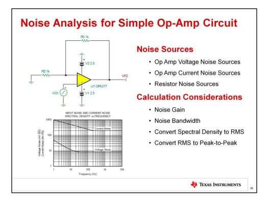
The noise analysis will involve looking at op amp noise voltage sources, op amp noise current sources, and resistor noise sources. The gain and bandwidth limitations of the op-amp will also effect the total noise calculation.
