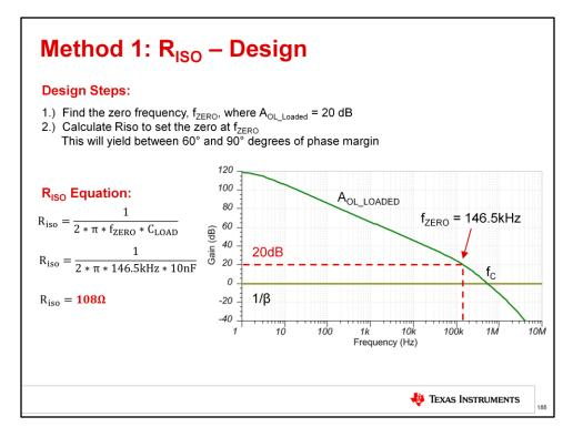
To design the Riso circuit for between 60 and 90 degrees of phase margin (depending on the op amp unity-gain phase margin and location of the Aol pole), first find the frequency where the Loaded Aol curve is equal to 20dB, f(Aol = 20dB). Using the Riso equations shown on the left and plugging in the values for Cload and f(Aol = 20dB), the Riso value is calculated to be 108  $\Omega$  in this example.
