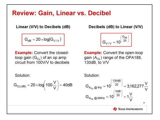
When working with electronics we often need to express quantities such as op amp gain, signal-to-noise ratio, common-mode-rejection ratio, and power supply rejection ratio whose values have very large spans.
