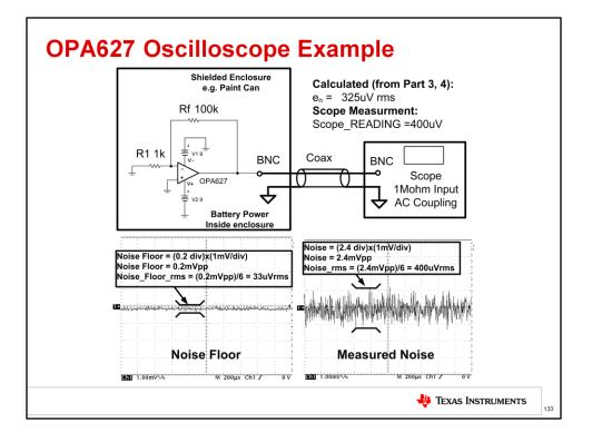
Let's now apply all of these real-world techniques to the OPA627 example circuit from our hand calculations and simulations. This circuit was connected directly to an oscilloscope with a BNC cable. As previously mentioned, the direct BNC connection is better than a 10x scope probe because the noise floor is ten times better.
