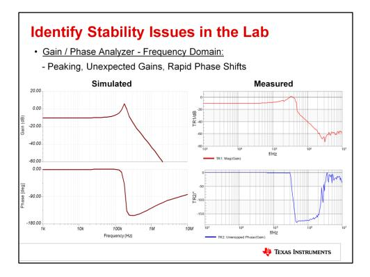
In addition to oscilloscopes, gain/phase analyzers can be used to measure the frequency response of a circuit which can also be used to identify stability issues. These results compare a circuit's simulated gain/phase response versus the measured response.
