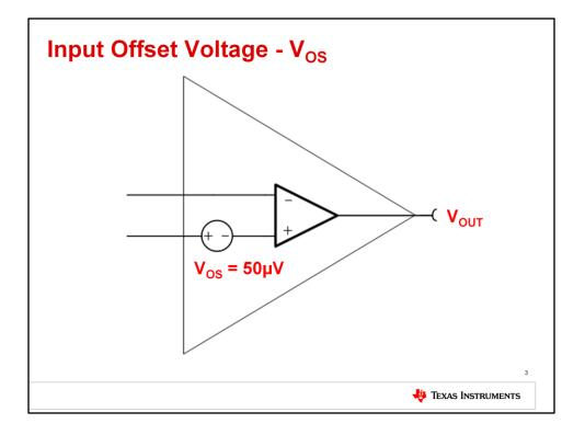
Let's start by defining offset voltage. Offset voltage is the differential input voltage that would have to be applied to force the op amp's output to zero volts. Typical offset voltages range from mV down to  $\mu$ V, depending on the op amp model. Offset can be modeled as an internal dc source connected to the input of the op amp. Changing power supply voltage and common mode voltage will affect input offset voltage.
