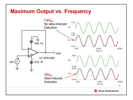
Let's simulate the conditions of the previous slide. With 7.5Vpk output, the response is sinusoidal with minimal distortion. However, with 10Vpk output, in a condition outside the full power bandwidth curve, the device is slew-rate limited and the output distorts.
