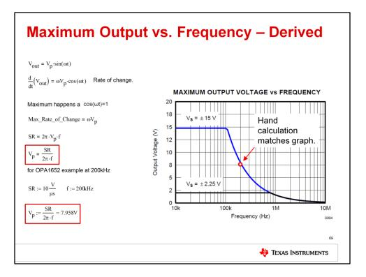
This slide illustrates that the maximum output vs. frequency curve can be derived with calculus. You can go through the math on your own, but the key point is that the final equation, Vpk = SR / (2 PI f) can be used if this curve is not available. The example shown in red confirms that the equation yields the same result as the curve.
