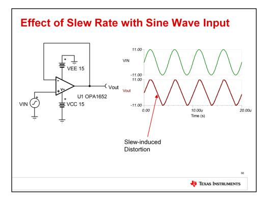
The slew rate of an op amp also impacts sinusoidal signals. If the op amp attempts to swing its output voltage past a certain frequency and amplitude which exceed the slew rate, the output will become distorted and will start to look more like a triangle wave. This limitation is called the full power bandwidth of the op amp.
