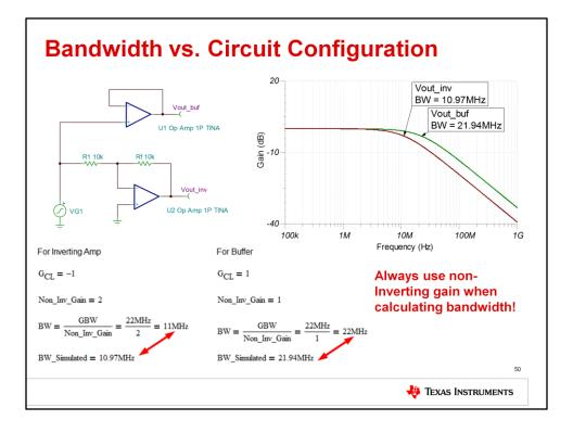
Earlier we calculated closed loop bandwidth for a non-inverting configuration using the gain bandwidth product. You might be surprised to learn that the bandwidth calculation for the *inverting* configuration is calculated using the *non-inverting gain*. Note that the non-inverting gain is typically referred to as noise gain.
