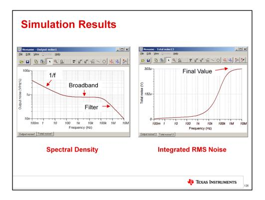
This slide shows the simulation results. The graph on the left is the spectral density plot, called "Output Noise" by TINA-TI. Note that the 1/f, broadband and filtered regions are clearly visible. The filtered region results purely from the op amp's inherent bandwidth limitations, since there is no filter on the circuit.
