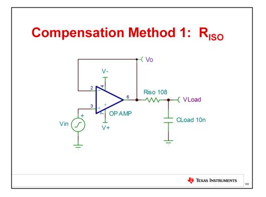
The Riso method is quite simple. It works by adding a zero to the Aol curve to cancel the pole from Ro and Cload.
