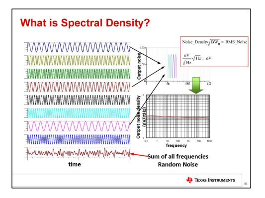
Do you remember that white light is the combination of all colors? Well, white noise is the combination of all frequencies. This figure shows that when you add several signals of different frequencies together in the time domain, the result is a random looking signal. In the frequency domain, each one of these signals looks like an impulse. Combining an infinite number of these signals across all frequencies creates what is called a noise spectral density curve.
