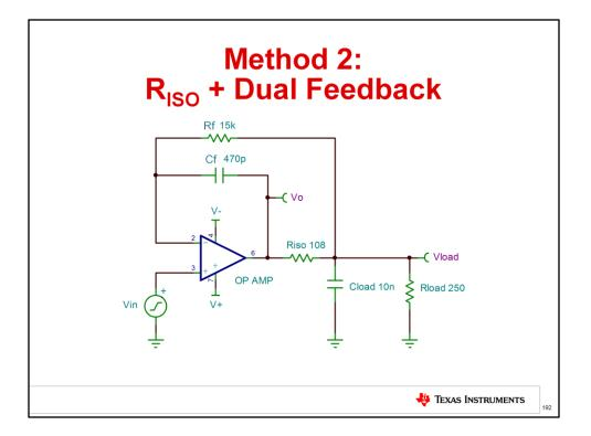
A solution to the voltage drop problem from the Riso circuit is to implement the "Riso + Dual Feedback" circuit shown here.
