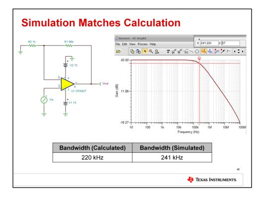
Let's now verify our bandwidth calculation with simulation. For the results to match, we must use the OPA827 in a non-inverting gain of 100V/V, or 40dB, like we did in the calculation on the last slide. If we run an AC transfer characteristic in TINA-TI, we see that the -3dB bandwidth, which occurs at 37dB since our DC signal gain is 40dB, is 241kHz. This matches well with our calculated bandwidth of 220kHz.
