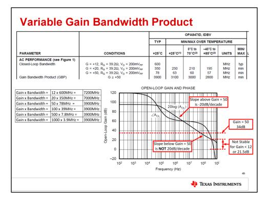
This slide shows the Aol curve for the OPA847, whose gain bandwidth product is defined for only a portion of the Aol curve. In this case it's defined only for closed loop gains greater than 50V/V.
