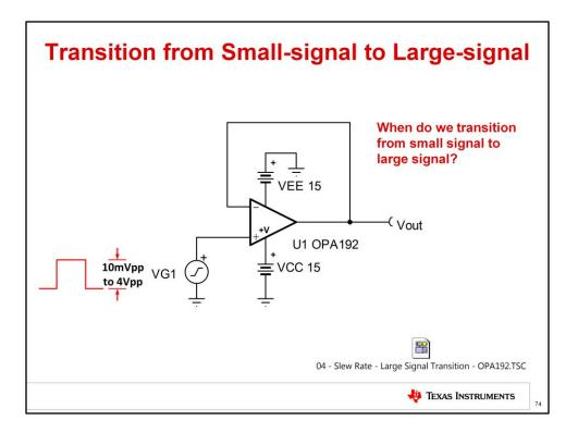
An amplifier's small-signal or large-signal behavior, like most things in the real world, isn't fully black and white. The way in which a circuit operates is not always fully large-signal or small-signal. In fact, there's a gradual transition between these two operating conditions.
