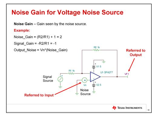
A key concept that we must understand before doing a noise analysis is **noise gain**. Noise gain is the gain seen by the noise voltage source, which is always on the noninverting input of the amplifier. It can be different from the signal gain. The example above shows a circuit with a noise gain of 2 and a signal gain of -1. In other words, the circuit is an inverting amplifier with respect to the signal source, but a noninverting amplifier to the noise voltage source.
