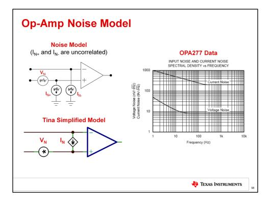
This slide show the typical op-amp noise model. In some cases, it is important to have two separate current noise sources, as shown in the upper left. In other cases, the simplified model with a single noise source between the inputs is adequate. The noise sources represent the spectral density curves. In the following lecture discussing noise, we will learn how to use the op amp noise model to predict the total peak-to-peak output noise for different amplifier configurations.
