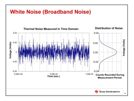
This slide shows the time domain waveform for white noise, also known as broadband noise. The time domain waveform is what you would see if you measured noise with an oscilloscope. Notice that the horizontal axis is 1ms, full scale. Taking the reciprocal of the full-scale time gives a frequency of 1kHz. In general, broadband noise is considered to be in the middle to high frequency range; that is, frequencies greater than 1kHz. In the next slide we'll consider lower frequency noise sources.
