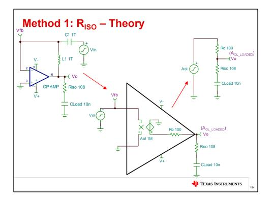
We can look at the Riso circuit the same way we looked at the original circuit. Here we see another voltage divider on the Aol output. This time there are two elements, Riso and Cload, on the bottom of the divider and Ro on the top leg of the divider.
