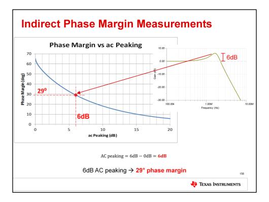
In AC Gain/Phase plots, the amount of ac peaking relative to the DC gain can be used to indirectly measure the phase margin of a circuit. In this example, the AC transfer function is peaking at 6dB, while the DC gain is 0dB. A total peaking of 6dB again results in 29 degrees of phase margin.
