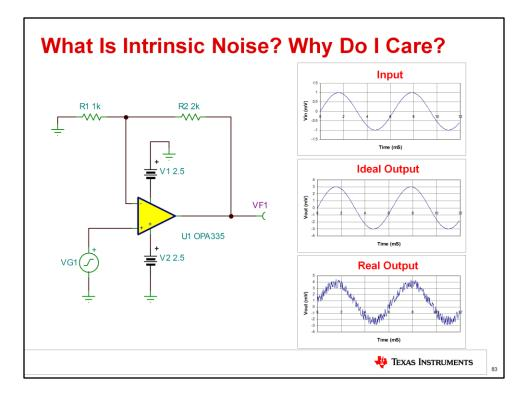
Noise can be defined as an unwanted signal that combines with a desired signal to result in an error. In audio, for example, noise can be noticed as a hiss or popping sound. In a sensor system, noise can be an error in the measured sensor output, such as pressure or temperature.
