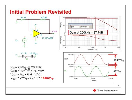
Let's return to our original problem, now that we understand the fundamentals of bandwidth. We have a non-inverting amplifier circuit with a closed-loop gain of 100V/V, or 40dB. The input is a 2mVpp sine wave at a frequency of 200kHz.
