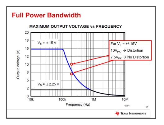
The graph above shows the maximum output sinusoidal waveform that can be generated without slew-induced distortion. This example considers a 200kHz signal at both 7.5Vpk and 10Vpk. At 7.5Vpk, the output signal is under the curve and therefore will not be distorted by slew rate limitations. At 10Vpk, the output signal is above the curve and will be distorted by slew rate limits.
