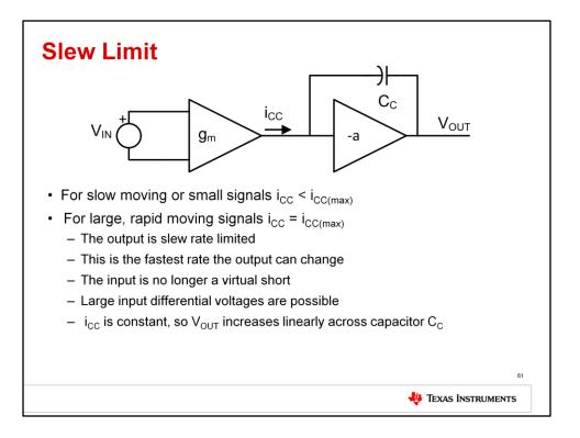
This is important with respect to slew rate of an amplifier. An amplifier has an internal  $g_M$ , or transconductance, stage which takes the input differential voltage and converts it to an output current,  $I_{CC}$ .  $I_{CC}$  flows into the next stage where it is used to charge  $C_c$ , which is called the Miller capacitance. If  $I_{CC}$  is a constant, then the voltage across  $C_c$  will rise linearly with time, just like we discussed on the previous slide.
