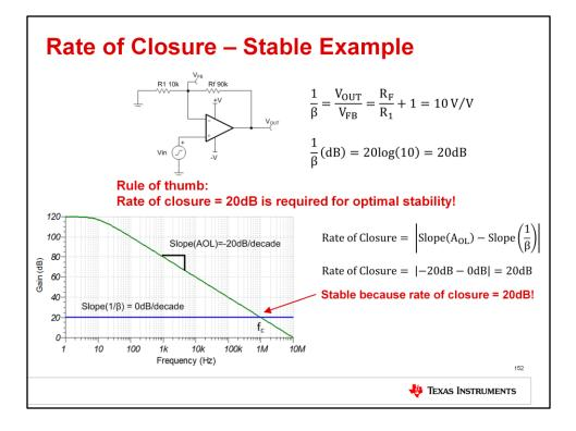
We can also analyze this circuit from earlier in the lecture using the rate of closure method. In this case, there is no capacitor in the feedback network, so there is no zero and therefore no increase in 1/B. Aol is still decreasing with a slope of - 20dB/decade as before. The rate of closure is now the absolute value of -20dB – 0dB, or 20dB. We can conclude that this circuit is stable.
