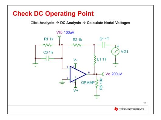
Before checking the AC behavior of the circuit, a quick check of the DC operating point should be done. Simply click Analysis, DC Analysis, and Calculate Nodal Voltages to do this. Vfb should show the input offset voltage, or Vos, of the op amp, while Vo will show Vos multiplied by the closed-loop gain.
