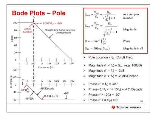
This slide is a review from the lecture on op amp bandwidth. It illustrates the equations for a pole and its associated magnitude and phase response on Bode plots. A pole causes a negative 20 dB/decade decrease in the slope of the magnitude response after the pole frequency, fp. The pole also causes a negative 90 degree phase shift in the phase response beginning roughly a decade before fp and ending roughly a decade afterwards.
