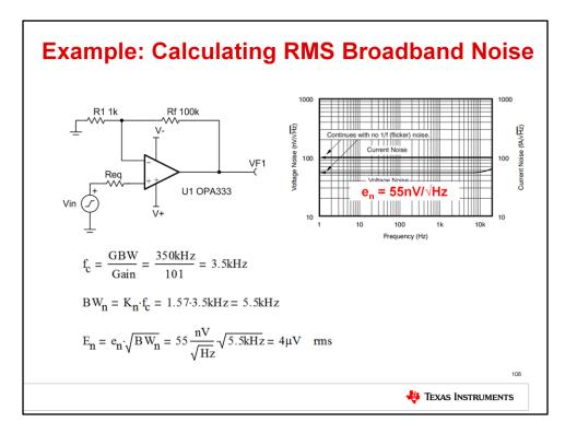
Let's continue the example calculation and determine the RMS broadband noise. The noise bandwidth from before is 5.5kHz. We now take the OPA333 input voltage noise spectral density and multiply it by the square root of the noise bandwidth to get a result of 4uVrms.
