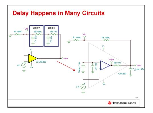
While the op amp circuit with the RC delay elements in the feedback path looks strange and unrealistic, many standard op amp circuits inadvertently create the same situation when external circuit components interact with non-ideal op-amp properties.
