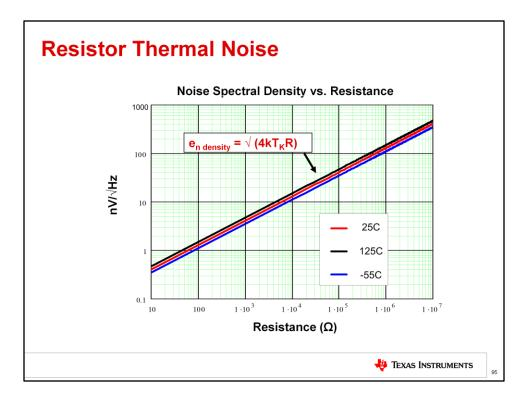
This plot was generated using the equation given in the last slide. Note that the equation was divided by the square root of bandwidth to give a spectral density, which is useful because it provides a quick way of comparing resistor noise to op-amp noise. Remember, most op-amps specify noise in nV/V(Hz).
