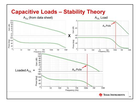
If the original op amp Aol curve and the Aol load curve are combined, the result is the loaded Aol curve shown on the bottom. As shown, the pole from the interaction of Ro and Cload causes a change to a -40dB/decade Aol magnitude slope and a degraded unity-gain phase margin.
