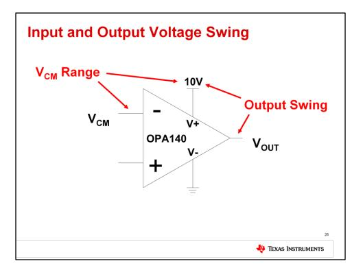
Common mode input voltage range is also known as input voltage swing. This term describes the range of input common mode voltages that can be used for normal linear operation of the amplifier. The common mode input voltage range is always defined relative to the positive supply and the negative supply. When you exceed the common mode input range, the output becomes nonlinear.
