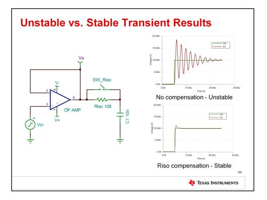
Comparing the transient response of the circuit both with and without Riso compensation, we can see the significant improvement by using Riso. Without Riso, the output of the circuit shows heavy overshoot and ringing.
