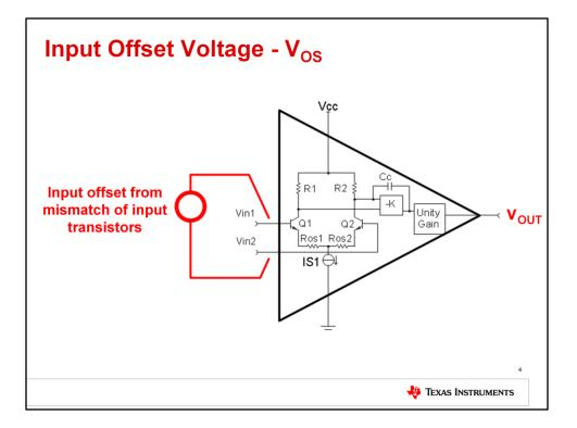
Looking at the inside of an op amp, we can see that the mismatch of transistors  $Q_1$  and  $Q_2$  in the differential input pair is what causes the offset voltage. In some cases, internal resistors  $R_{OS1}$  and  $R_{OS2}$  are laser trimmed in order to compensate for this mismatch and obtain very low offset voltage. In other cases, an internal digital correction circuit is used to minimize offset voltage and offset drift.
