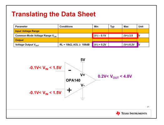
Let's look at how common mode voltage and input and output voltage swing are typically defined on a data sheet.
