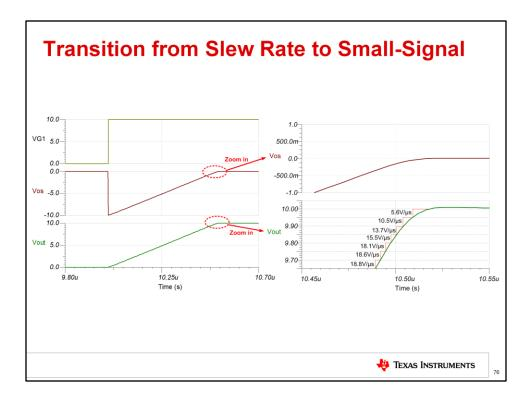
Let's take a closer look at the output of the non-inverting buffer circuit with a 10V step applied to the input.
