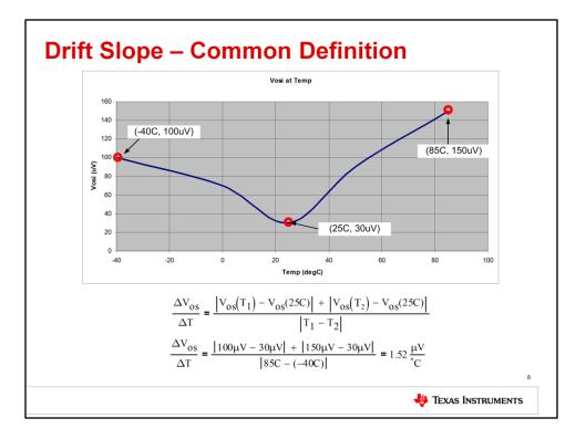
This is the more common definition for drift, which is separated into different two regions, although more than two regions could be used if desired.
