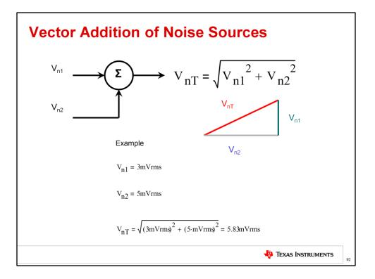
An important concept in nose analysis is adding noise values. Noise cannot be added algebraically, for example, 3+5=8. Noise must be added as a vector as shown here, where we take the square root of 3mVrms squared plus 5mVrms squared for a result of 5.83mVrms. It is important to note that this relationship applies only to uncorrelated ,random noise. If the noise source is correlated, a different formula applies.
