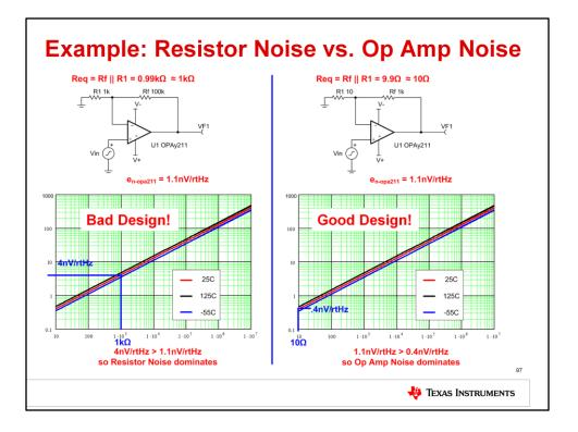
Let's compare resistor/thermal noise to op amp noise in two different circuits.
