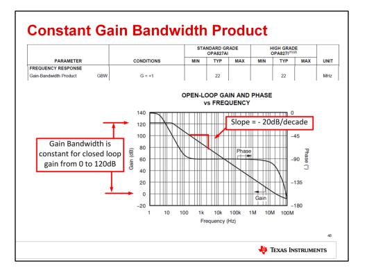
In this slide we further examine the OPA827 open loop gain curve. We see that the dc open loop gain is 120dB and remains constant until we reach the dominant pole. At frequencies greater than the dominant pole, the open loop gain decreases at a rate of -20dB per decade. Notice that for the OPA827 the slope of Aol is constant until we cross unity gain. Therefore the gain bandwidth product is constant for closed loop gains from 0 to 120 decibels.
