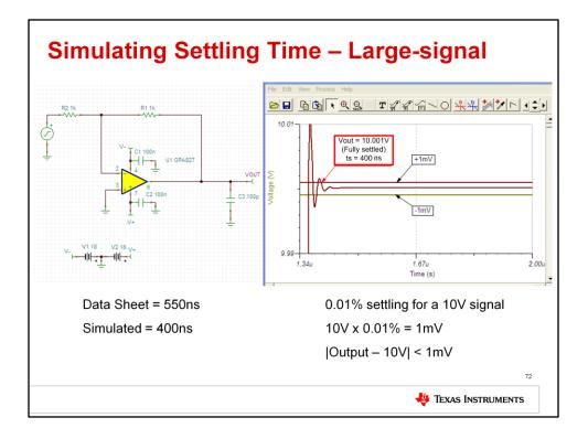
The settling behavior, with some overshoot and damped oscillations, can really be seen once we zoom in on the plot. In this example, the output settles after an over shoot and one cycle of ringing, for a total settling time of 400ns. This is acceptably close to the typical data sheet value of 550ns.
