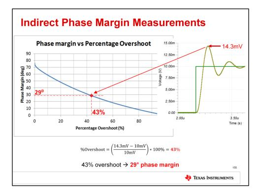
In the time domain the percent overshoot to a step input can be used to indirectly calculate the phase margin. In this example, a 10mV step was applied. The output overshoot reached 14.3mV, or 4.3mV above the intended output. This corresponds to a percent overshoot of 43%. Using the phase margin vs. percentage overshoot plot, we can see that 43% of overshoot results in only 29 degrees of phase margin.
