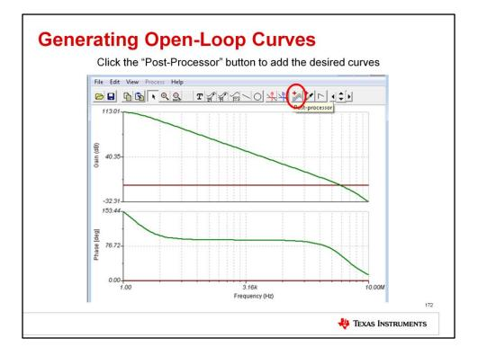
TINA by default will only display the curves which have markers, which in this example is Vo and Vfb. To add the desired curves for open-loop analysis, click the post-processor button in the result window.
