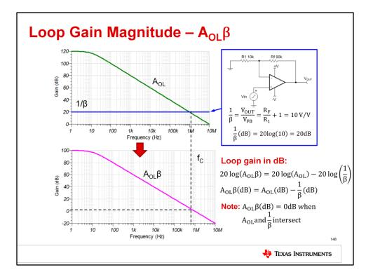
Well, first we can consider the loop gain magnitude using a Bode plot. Using the same circuit as before, we have a gain of 10V/V, or 20dB, so 1/B is a constant 20dB over frequency. The circuit's Aol is also shown. To find the magnitude of AolB, we can simply subtract 1/B from Aol. This might not seem intuitive, but the mathematical relationship shown on the right side of the slide proves this using the properties of logarithms.
