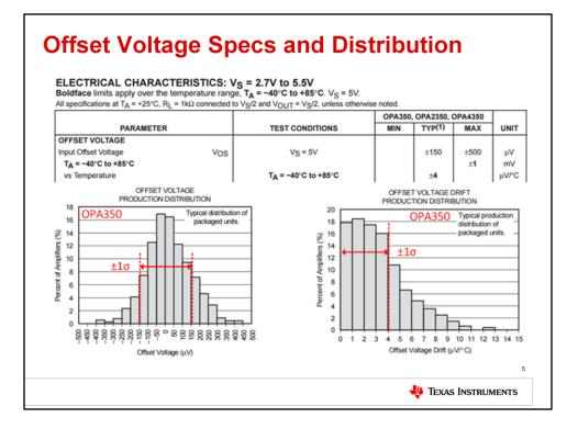
This slide introduces op amp specifications. The top of the specification table is the test conditions for all the parameters in the data sheet. In this example, the temperature is 25 °C, the load resistance is  $1 k \Omega$ , the load is connected to mid supply, and the common mode voltage is set to mid supply. These conditions are true unless otherwise specified. If you look at the offset voltage specs, it lists some additional conditions. The supply voltage is 5V.
