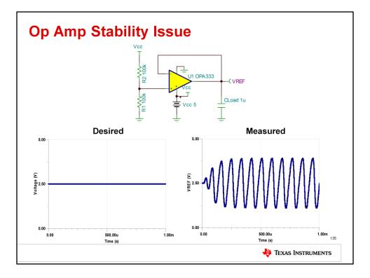
Here is an example of what can happen if a circuit's stability is not verified before going to production. An op amp circuit that is unstable will have an unpredictable or unexpected output with poor transient performance. This typically results in large overshoots and ringing when changes occur on the input or load, but may also result in sustained oscillations. Often stability problems are caused by connecting a capacitor to the output or to the inverting input of the amplifier.
