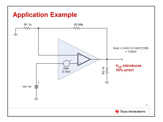
In this application example we will see how to calculate the output voltage error from the offset voltage.
