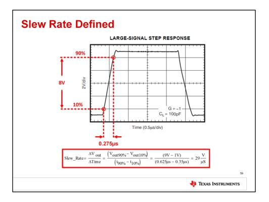
Slew rate is defined as the maximum rate of change of an op amp's output voltage and is given units of volts per microsecond. Slew rate is measured by applying a large signal step, such as 1V, to the input of the op amp, and measuring the rate of change from 10% to 90% of the output signal's amplitude.
