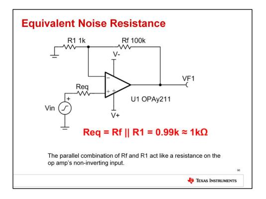
For noise calculations, it is often necessary to calculate Req, the equivalent resistance seen by the input. The most common method for calculating Req is given here. The parallel combination of Rf and R1 act like a resistance on the op amp's non-inverting input, so Req in this example has a value of approximately 1k.
