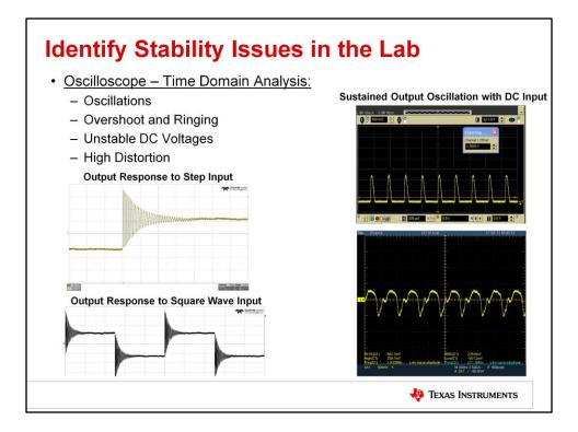
Here are some images of output signals from unstable circuits taken with common lab oscilloscopes.
