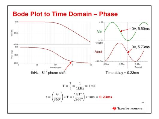
Here we will continue the example considering the phase shift in the time domain. Notice on the **bode phase (Phase (deg))** that the phase shift is -81degrees at 1kHz. On the time domain plot, you can see that the output signal is shifted to the right in time. This is called a phase shift or time delay. The calculation at the bottom of the page illustrates how you can convert the phase shift in degrees to expected time delay in seconds.
