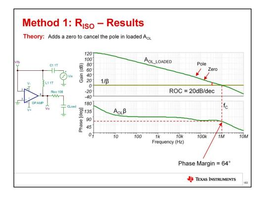
Looking at the open-loop results from the "Riso" compensation method, a zero can be seen cancelling the pole from Riso and Cload. This results in a return to a 20dB/decade Aol slope and significantly improved phase margin.
