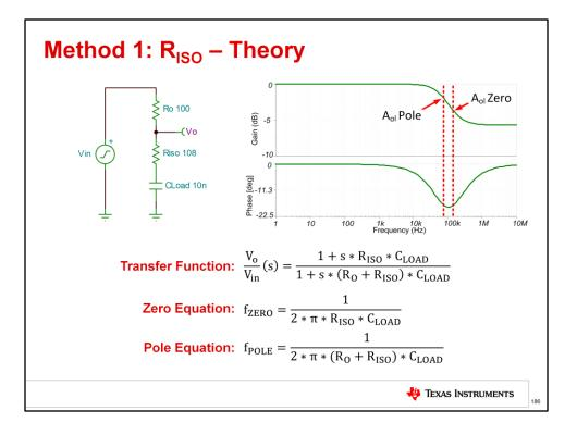
The resulting Laplace transfer function for this circuit is shown here. Again, with a single "s" term in both the numerator and denominator it is clear that there is now both a pole and a zero in the transfer function. The equations for the pole and zero frequency can be calculated from the transfer function. Plotting the AC transfer function, you can see that the positive phase shift from the zero cancels the negative phase shift from the pole, causing a net phase shift of zero degrees.
