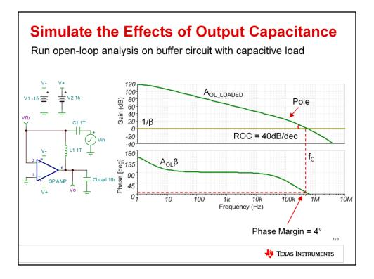
Using the steps shown previously, we ran an open-loop simulation on the circuit shown here with a 10nF capacitor on the op amp output. As the results show, the 10nF capacitive load results in a pole in the Aol curve which degrades the Aol\*ß phase to only 4 degrees at fc. Let's examine why this happens.
