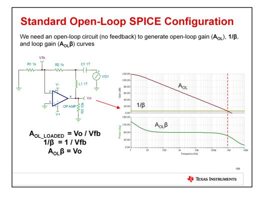
In order to successfully generate the open-loop curves to perform the rate-of-closure and phase margin analysis, the feedback loop of the op amp needs to be broken. Then, a small signal source can excite the high-impedance node of where the loop was broken and measurements can be taken at the input (Vfb) and output (Vo) to derive the desired curves.
