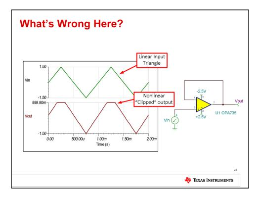
Lets start by considering this simple non-inverting buffer circuit. An triangle-wave input signal of +/- 1.5V is applied to the non-inverting input, and one might expect the output to look exactly the same. For some reason, the op amp output does not increase past +1V. This type of nonlinearity is called "clipping."
