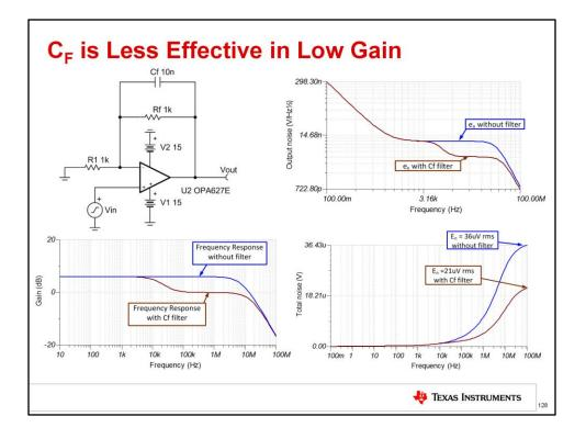
In this example the closed-loop gain is 2V/V or 6dB. The filter behaves in the same way, except that the effective attenuation when the capacitor is acting like a short is only 6dB. In general, this type of filter will reduce the gain from the dc gain to a gain of 1V/V. Thus, this filter is most effective for circuits with high gain.
