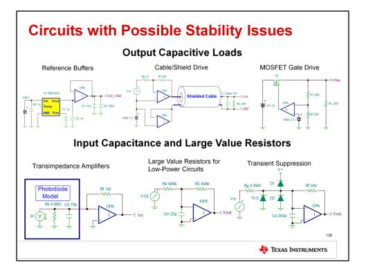
So, without further ado, here are the most common circuits and applications involved in op amp circuit stability issues. These circuits all create unwanted delay from the output to the feedback node and can be divided into two distinct groups based on the issue they cause in the op amp control loop.
