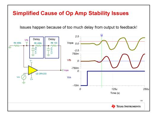
Too much delay between the amplifier output and the inverting feedback node is a straightforward way to visualize the root cause of op amp stability issues.
