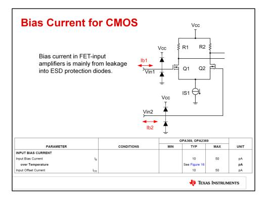
In the case of MOSFET or JFET op amps, the input bias current is primarily due to the leakage of the input ESD protection diodes. The gate of the input MOSFET transistors has extremely low leakage, so it doesn't contribute significant bias current. You can see in this example that the OPA369 has 50pA max of input bias current.
