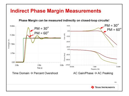
Phase Margin can also be indirectly measured on closed-loop circuits in the time domain and in ac gain/phase measurements. In the time domain, we can observe phase margin based on the overshoot of an op amp's output relative to a small-signal step input. In the frequency domain, we can observe phase margin based on the maximum AC peaking in the circuit's transfer function compared to the DC gain.
