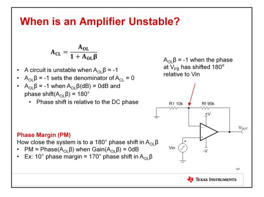
First, we must define when an amplifier is unstable. Looking back at the op amp closed-loop gain equation, we remember that Acl = Aol / 1+ AolB. Taking a closer look, we can see that if AolB, or the loop gain, equals -1, we get zero in the denominator and therefore Acl becomes undefined. This is the mathematical definition of instability. How can this happen in a real circuit?
