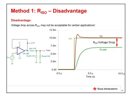
While the Riso circuit is both simple to implement and design it has a big disadvantage in precision circuits. The voltage drop from Riso is dependent on the output current or output load, and may be significant compared to the desired signal. As shown here a 10mV signal has over 3mV (30%) of error due to a 250 $\Omega$  output load.
