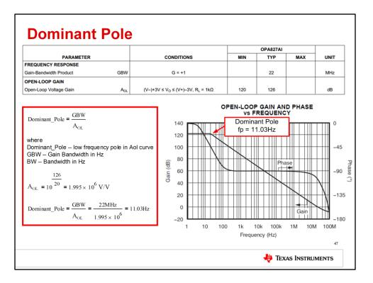
The dominant pole is the point on the Aol graph where Aol begins to roll off with frequency. This parameter is important when developing macromodels. The frequency of the pole can be estimated from the Aol curve, but a more accurate approach is to calculate it using this equation, where GBW is the gain bandwidth product and Avol is the open loop gain of the device.
