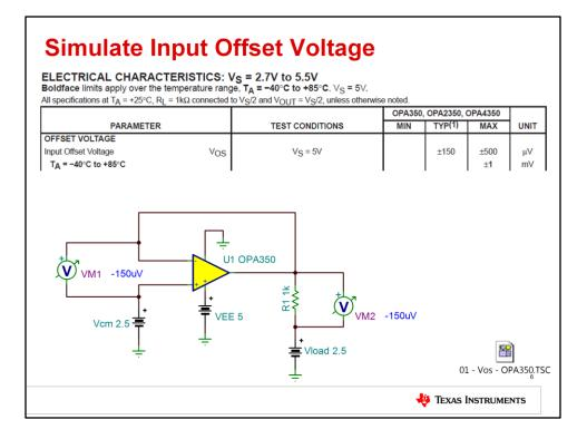
Most op amp SPICE models include the effects of offset voltage. Several external conditions, such as power supply voltage and common mode voltage, affect the offset voltage on a real world device. These effects are also included in the simulation model.
