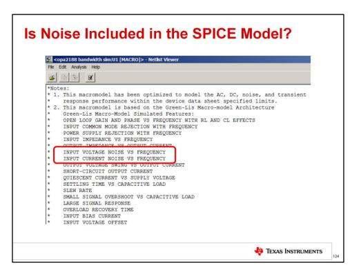
Another important thing to check before doing a simulation is if the op amp's SPICE model includes noise characteristics. If you double-click on Texas Instruments models in TINA-TI and click "Enter Macro," a net list viewer will open. The top of the net list on TI models includes a description of what is modeled. The key parameters to look for are **input voltage noise vs. frequency** and **input current noise vs. frequency**.
