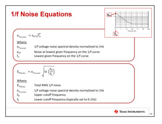
Let's move on to the 1/f noise equations. The first equation gives the 1/f noise normalized to 1Hz, given by  $e_{n\_normal}$ . This means that we take a point on the 1/f curve and translate the spectral density to a level corresponding to what would be read at 1Hz. In general, it is best to choose  $e_{nf}$  at the lowest frequency possible, because this will ensure that 1/f is dominant.
