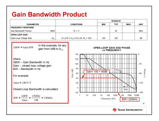
A simple approach to determining bandwidth is to use the gain-bandwidth product specification from an op amp data sheet.
