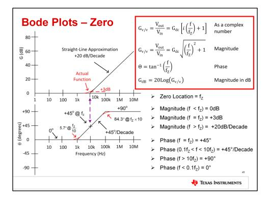
This slide illustrates the equations for a zero and its associated response. Looking at the equations, you can see that the first equation represents a zero as a complex number. Complex numbers have a real and imaginary part. For practical circuits the complex function is converted to a magnitude and phase. The second equation shows the magnitude and the third equation shows the phase. Taking 20 Log10 of the magnitude function gives the magnitude in dB.
