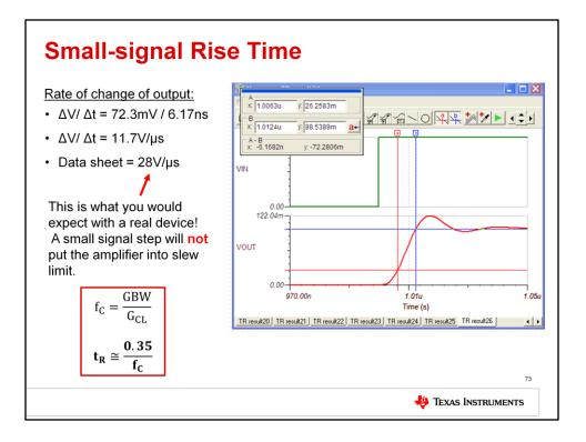
Here we observe the **small-signal** rise time of the same circuit, for purposes of comparison to the large-signal slew rate. Again, let's zoom in on the rising edge of the small signal step response. Measuring delta V over delta T from 10% to 90% of the output swing, me get a rise time of  $11.7V/\mu s$ . Compare this to the data sheet slew rate value of  $28V/\mu s$  – they're quite different!
