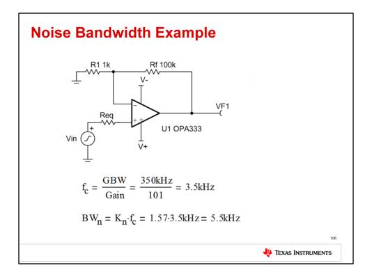
Let's calculate an example noise bandwidth for a simple circuit.
