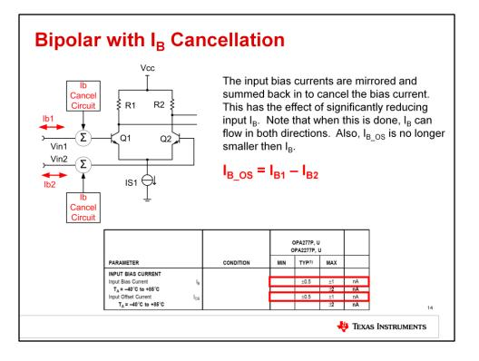
Some precision bipolar op amps use a method called bias current cancellation in order to minimize bias current. This is done inside the op amp, so no external components are required. The amplifier simply behaves like a bipolar amplifier with very low bias current.
