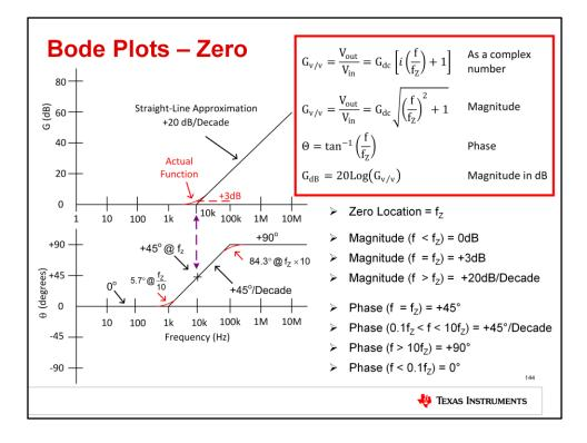
This slide, also from the op-amp bandwidth lecture, illustrates the equations for a zero and its associated magnitude and phase response on Bode plots. A zero causes a positive 20dB/decade increase in the slope of the magnitude response after the zero frequency, fz. The zero also causes a positive 90 degree phase shift in the phase response beginning roughly a decade before fz and ending roughly a decade afterwards.
