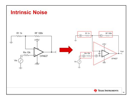
This slide illustrates how an amplifier circuit can be translated into a noise equivalent circuit.
