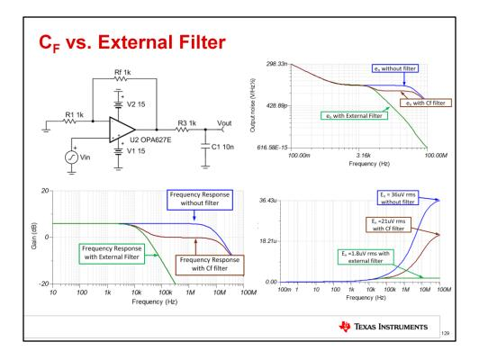
Using an external filter, which is a filter outside the op amp feedback loop, is the most effective way to reduce noise in circuits with low gain.
