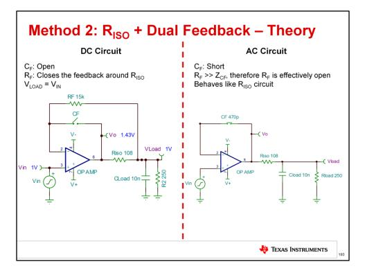
The Riso + dual feedback circuit works by having an equivalent circuit at both DC and AC.
