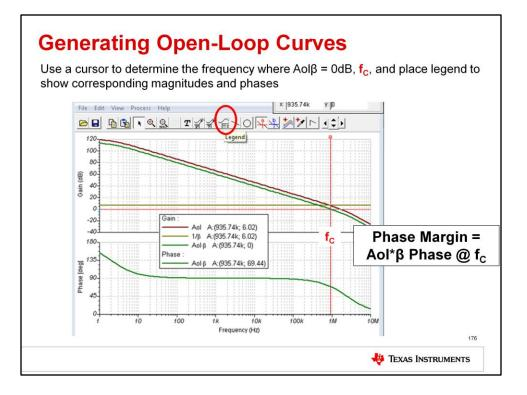
The final step is to measure the phase margin on the curves. The easiest method is to place a cursor on the Aol\* $\beta$  curve and then type "0" into the "y:" text box to set the cursor to the fc frequency. Then click the "Legend" button and place it on the screen, which will display the phase of Aol\* $\beta$  at fc. This is the phase margin.
