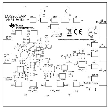
Figure 3-3. Top Overlay PCB Layout
