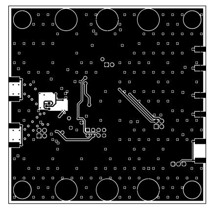
Figure 3-7. Bottom Layer PCB Layout
