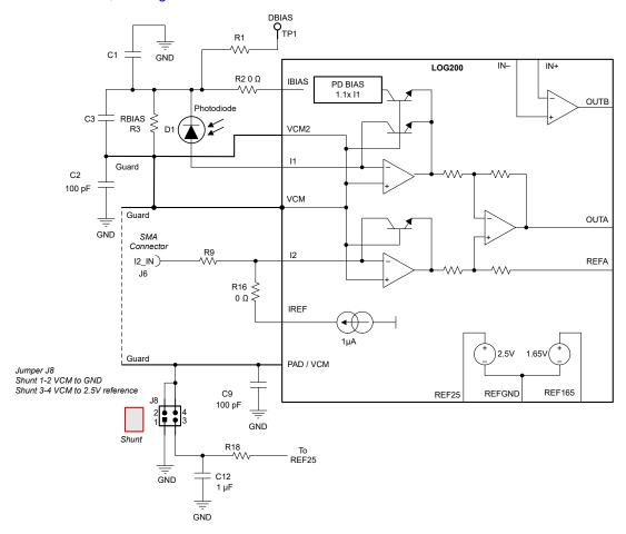
Figure 2-3. LOG200EVM Photodiode Connections
