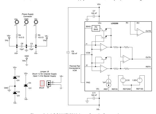
Figure 2-1. LOG200EVM Voltage Supply Connections
