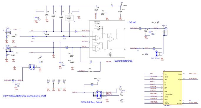
Rev E3: Modified REF25 connection to VCM, through REF25 filter: R18=100Ohm, C12=1uF. Modified Capacitors values C2, C9 from 1000pF to 100pF Modified REF165 bypass capacitor C14 from 330pF to 100pF. Added C19, R36, R37, R38, TP7 for flexibility.
