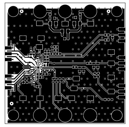
Figure 3-4. Top Layer PCB Layout
