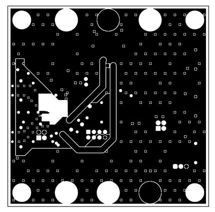
Figure 3-5. Mid Layer 1 PCB Layout
