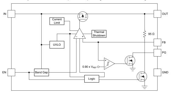
Figure 1-1. Adjustable Version With Open-Drain Power-Good
