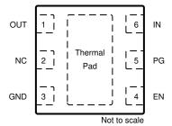
Figure 4-2. Pin Diagram (Fixed TPS746-Q1 DRV Package)
