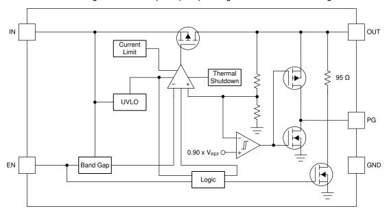
Figure 1-4. Fixed Voltage Version With Push-Pull Power-Good
