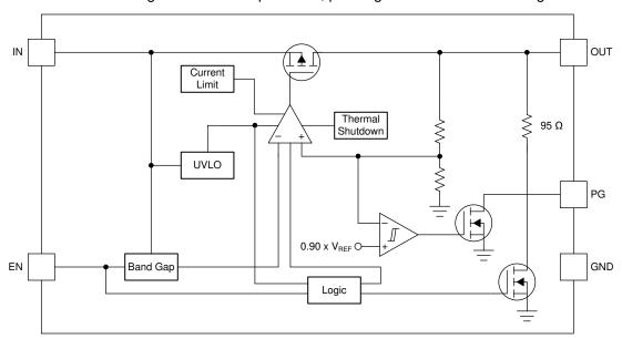
Figure 1-3. Fixed Voltage Version With Open-Drain Power-Good
