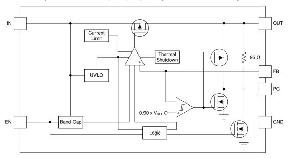
Figure 1-2. Adjustable Version With Push-Pull Power-Good
