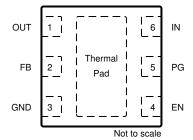
Figure 4-1. Pin Diagram (Adjustable TPS746-Q1 DRV Package)
