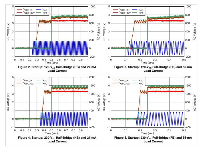
Figure 2 to Figure 5 show various start-up plots for the TPS7A78EVM-011.
