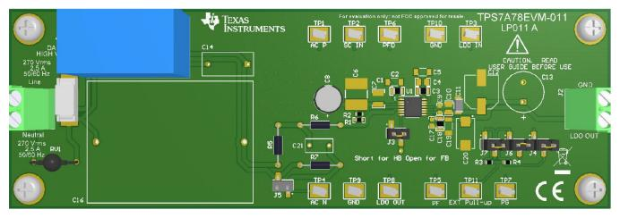
This user's guide describes the operational use of the TPS7A78EVM-011 evaluation module (EVM) as a reference design for engineering demonstration and evaluation of the TPS7A78, non-isolated smart linear voltage regulator (LDO). Included in this user's guide are setup and operating instructions, thermal and layout guidelines, a printed circuit board (PCB) layout, a schematic diagram, and a bill of materials (BOM).
