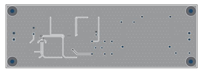
Figure 11. Bottom Layer Routing
