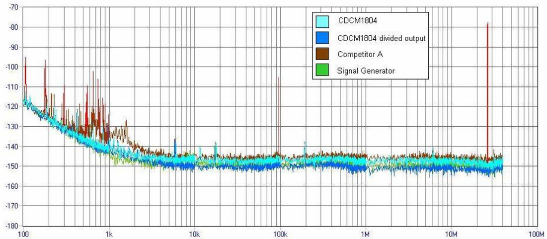
Figure 13. Phase Noise Plots of the CDCM1804 and Competitor A at 106.25 MHz, 2.5 V
