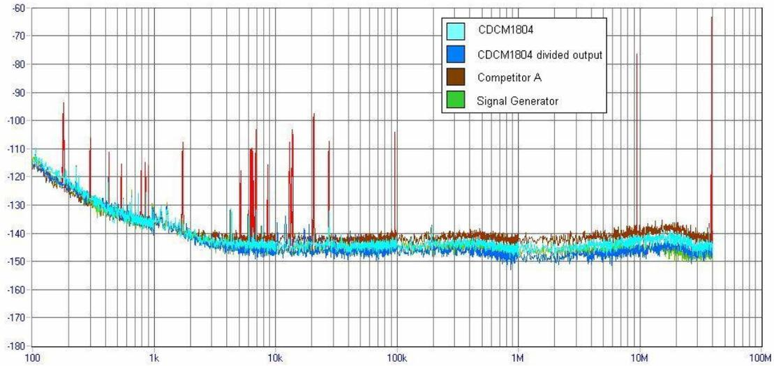
**Figure 10. Phase Noise Plots of the CDCM1804 and Competitor A at 156.25 MHz, 3.3 V**
