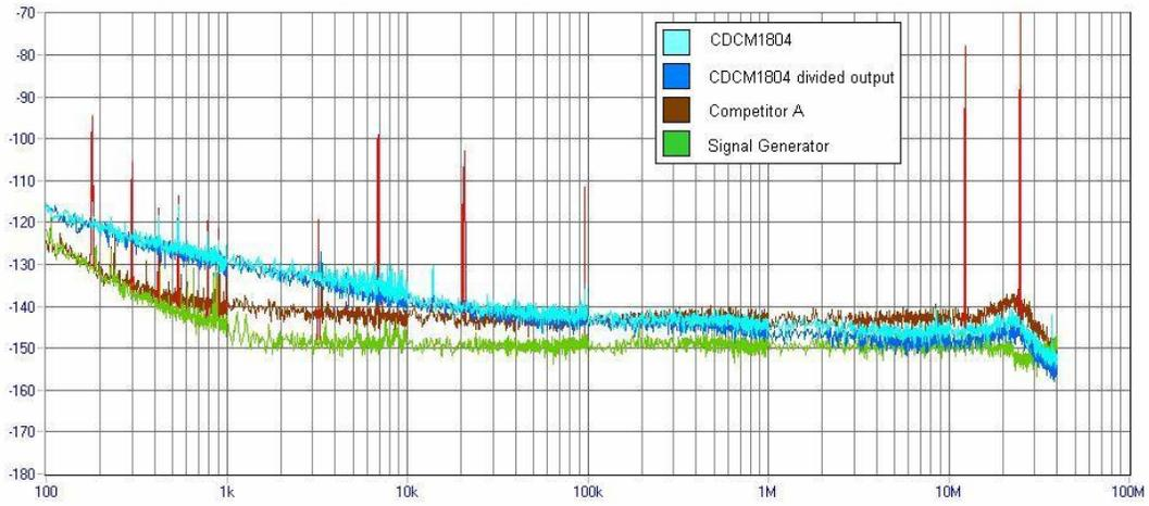
**Figure 8. Phase Noise Plots of the CDCM1804 and Competitor A at 50 MHz, 3.3 V**
