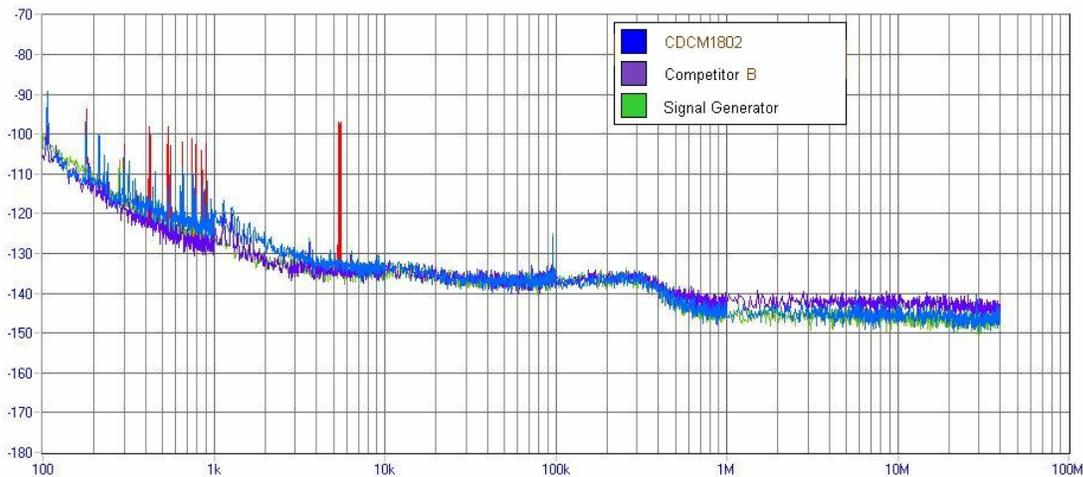
**Figure 23. Phase Noise Plots of the CDCM1802 and Competitor B at 622.08 MHz, 2.5 V**
