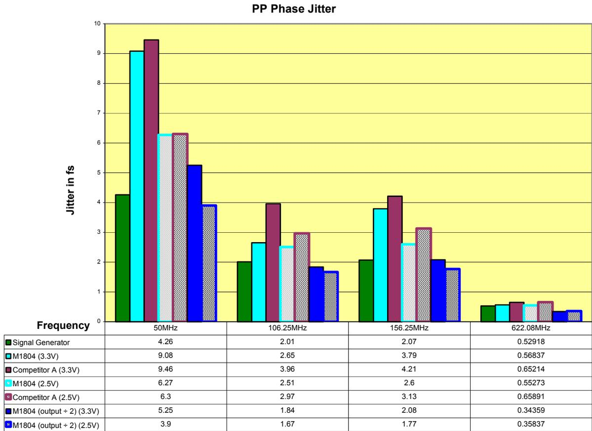
**Figure 3. PN9000 Peak-to-Peak Phase Jitter Measurements of the CDCM1804 and Competitor A**
