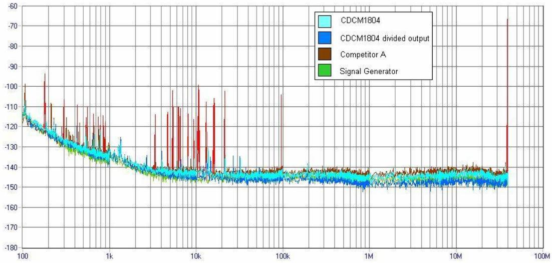
**Figure 14. Phase Noise Plots of the CDCM1804 and Competitor A at 156.25 MHz, 2.5 V**
