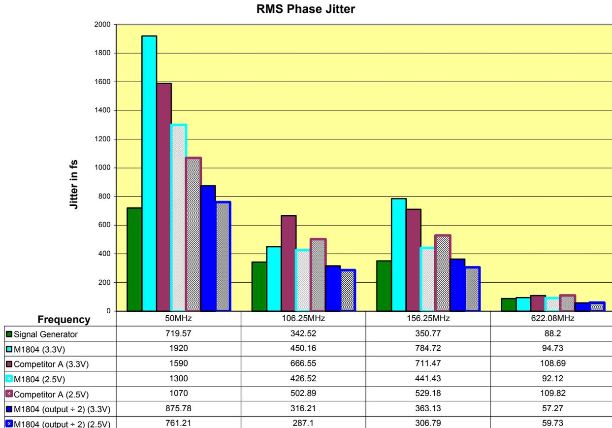
**Figure 2. PN9000 RMS Phase Jitter Measurements of the CDCM1804 and Competitor A**
