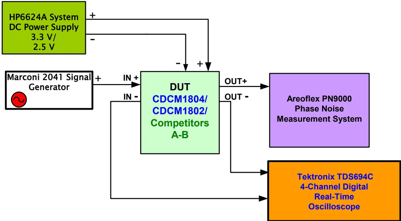
**Figure 1. Test Setup for Phase Noise Measurements Taken from the AeroFlex PN9000**
