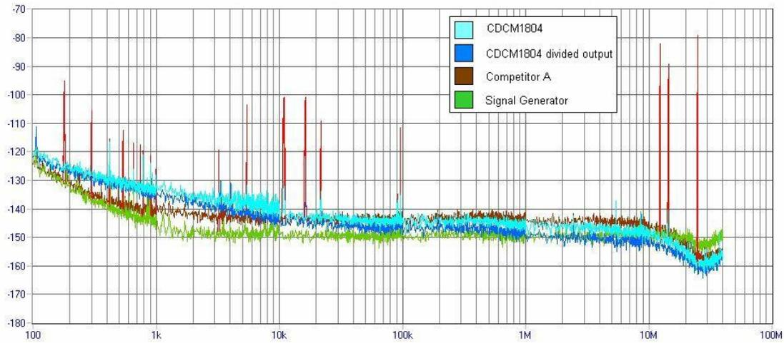
Figure 12. Phase Noise Plots of the CDCM1804 and Competitor A at 50 MHz, 2.5 V
