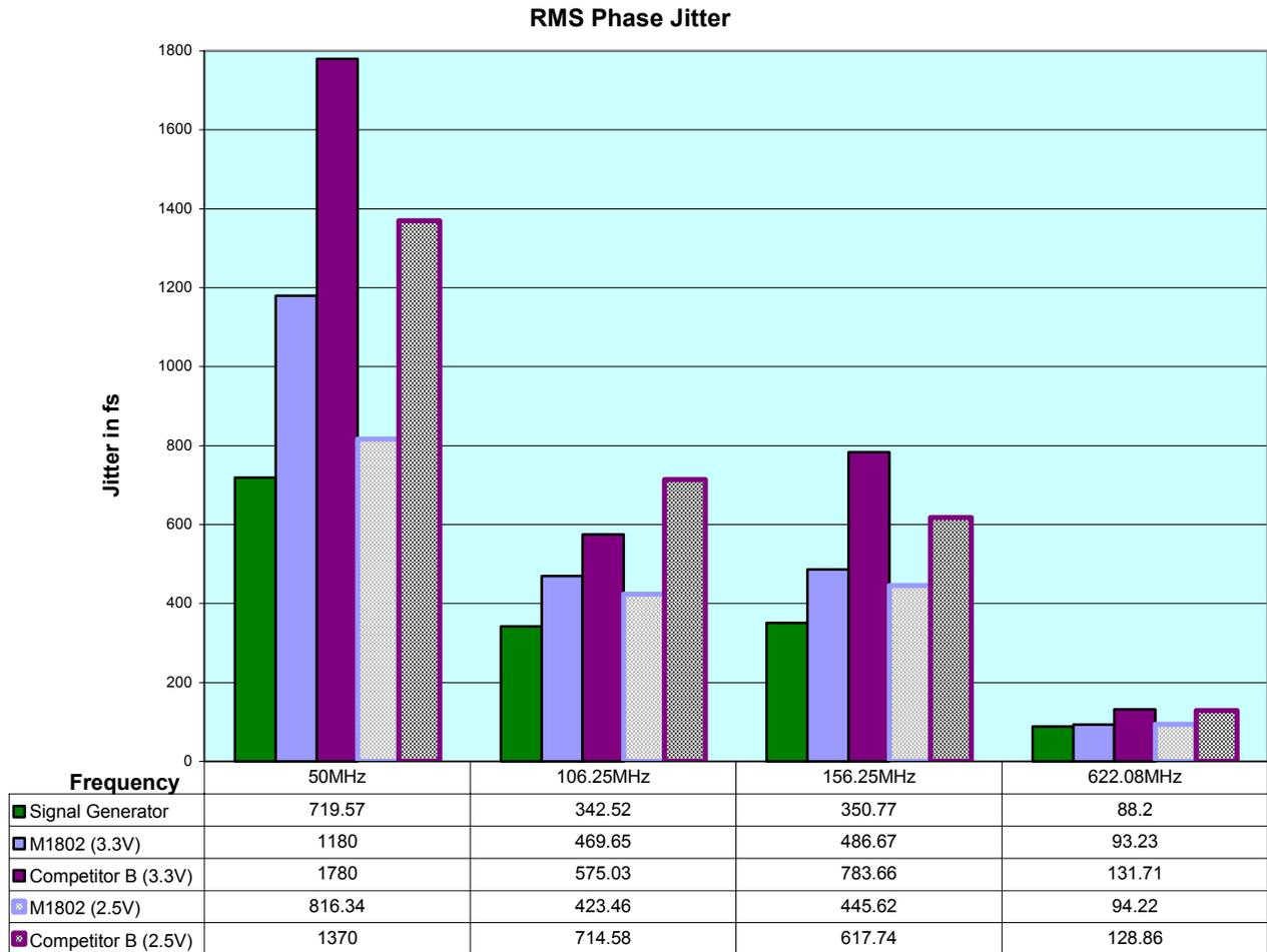
**Figure 5. PN9000 RMS Phase Jitter Measurements of the CDCM1802 and Competitor B**
