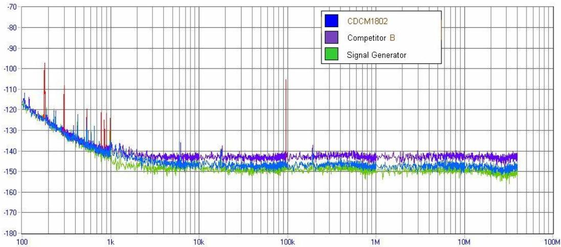
**Figure 21. Phase Noise Plots of the CDCM1802 and Competitor B at 106.25 MHz, 2.5 V**
