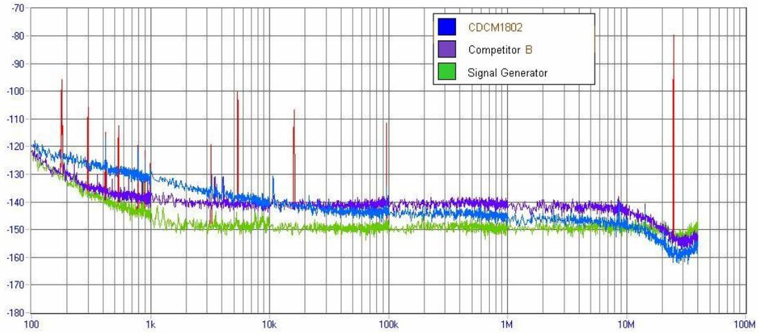
**Figure 20. Phase Noise Plots of the CDCM1802 and Competitor B at 50 MHz, 2.5 V**
