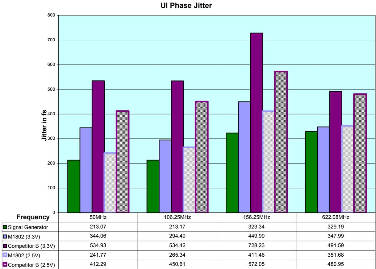
**Figure 7. PN9000 Unit Interval Phase Jitter Measurements of the CDCM1802 and Competitor B**
