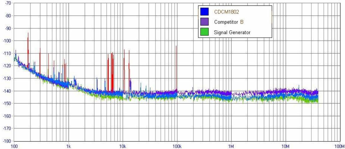
**Figure 22. Phase Noise Plots of the CDCM1802 and Competitor B at 156.25 MHz, 2.5 V**
