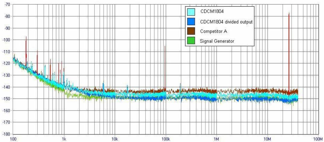
**Figure 9. Phase Noise Plots of the CDCM1804 and Competitor A at 106.25 MHz, 3.3 V**
