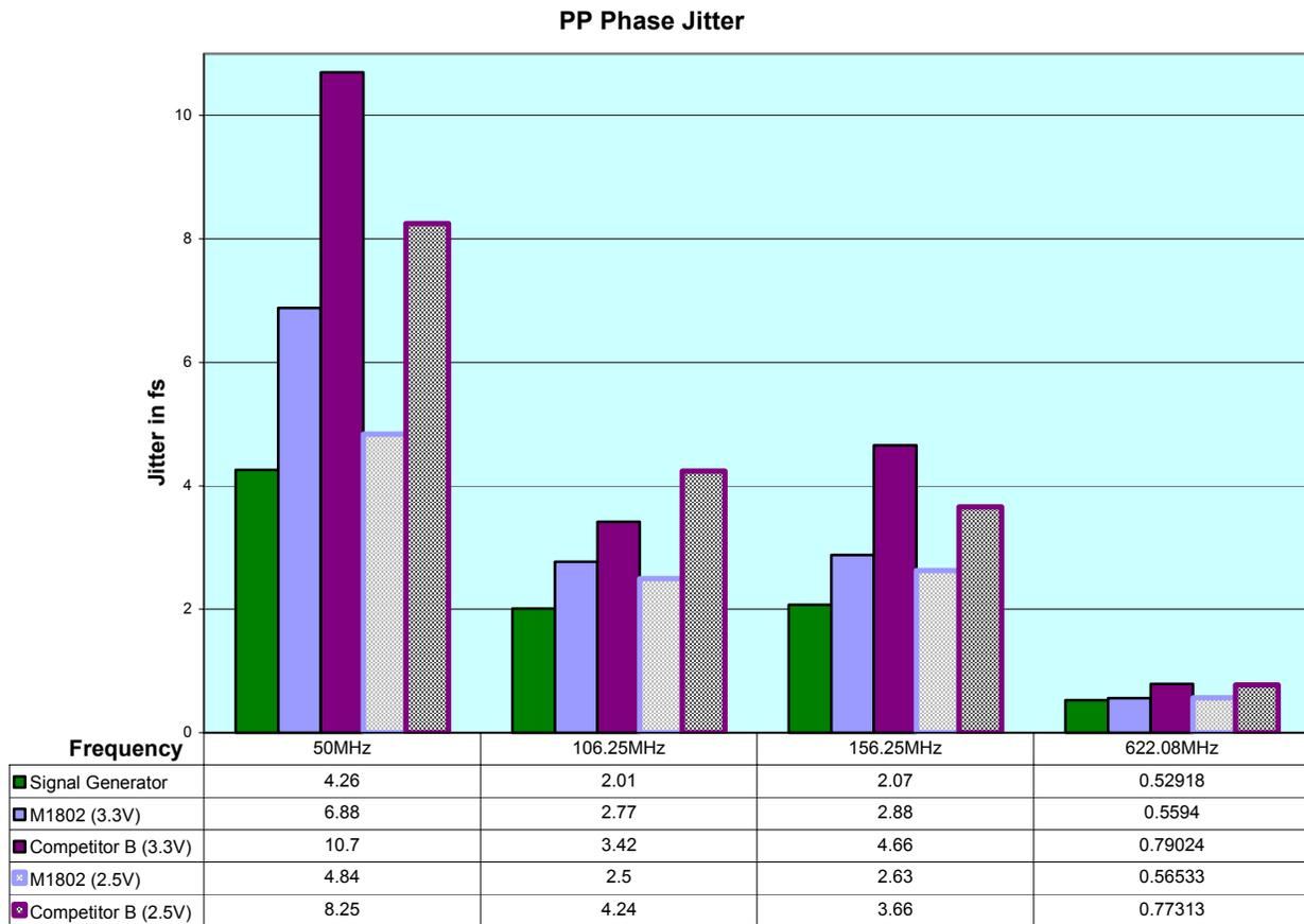
**Figure 6. PN9000 Peak-to-Peak Phase Jitter Measurements of the CDCM1802 and Competitor B**
