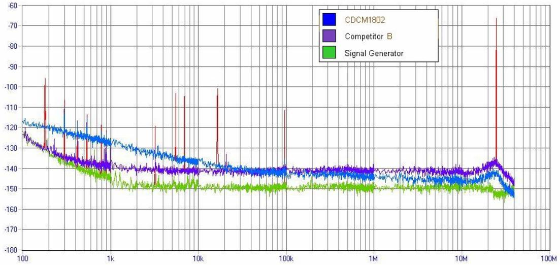
**Figure 16. Phase Noise Plots of the CDCM1802 and Competitor B at 50 MHz, 3.3 V**
