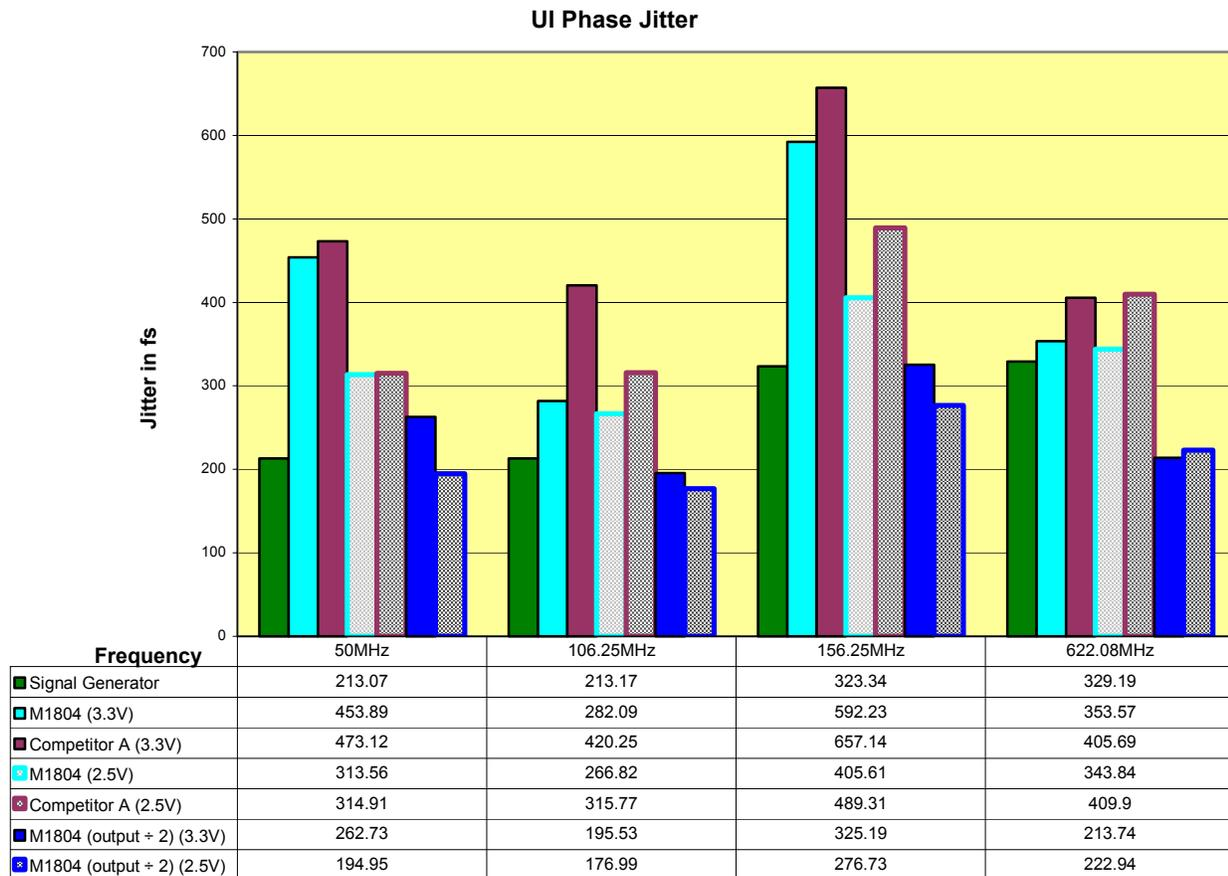
**Figure 4. PN9000 Unit Interval (UI) Phase Jitter Measurements of the CDCM1804 and Competitor A**
