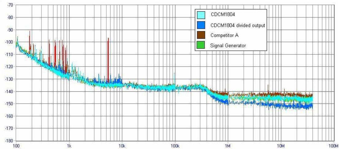
**Figure 11. Phase Noise Plots of the CDCM1804 and Competitor A at 622.08 MHz, 3.3 V**
