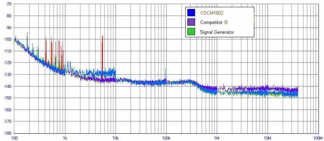
**Figure 19. Phase Noise Plots of the CDCM1802 and Competitor B at 622.08 MHz, 3.3 V**
