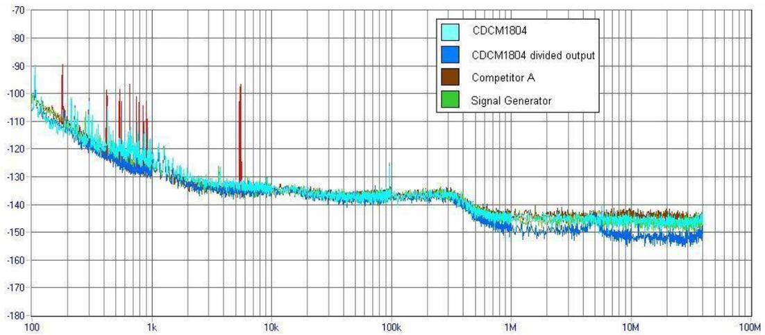
**Figure 15. Phase Noise Plots of the CDCM1804 and Competitor A at 622.08 MHz, 2.5 V**
