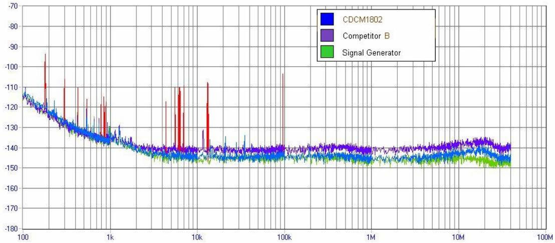
**Figure 18. Phase Noise Plots of the CDCM1802 and Competitor B at 156.25 MHz, 3.3 V**
