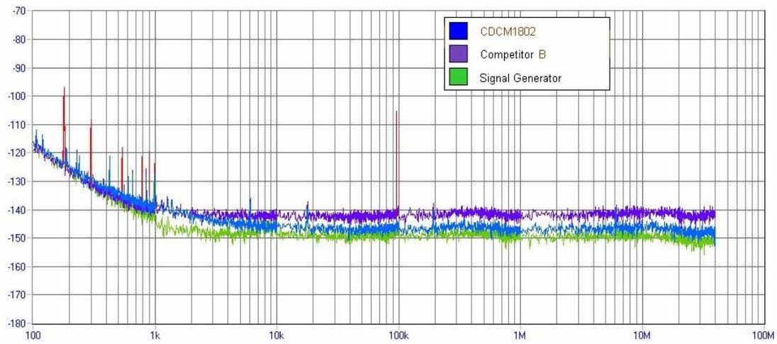
**Figure 17. Phase Noise Plots of the CDCM1802 and Competitor B at 106.25 MHz, 3.3 V**
