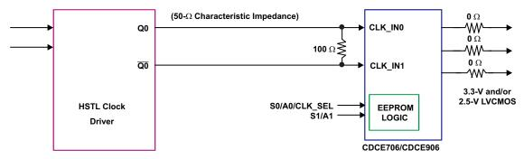
Figure 5. DC Coupling Between HSTL Driver and CDCE706/906
