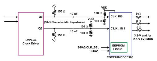
Figure 4. AC-Coupling Between LVPECL Driver and CDCE706/906
