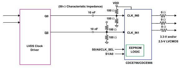
Figure 2. AC-coupling Between LVDS Driver and CDCE706/906
