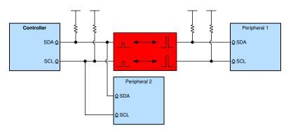
Figure 1. Example I2C Voltage Translation Block Diagram
