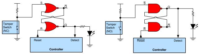
Figure 3-4. Using Logic to Monitor a Normally Closed (NC) Tamper Switch
