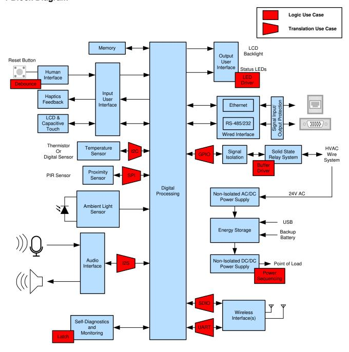
Figure 1-1. Simplified Block Diagram for Smart Thermostats
