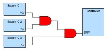
Figure 3-2. Using Logic to Combine Multiple Power-Good Signals
