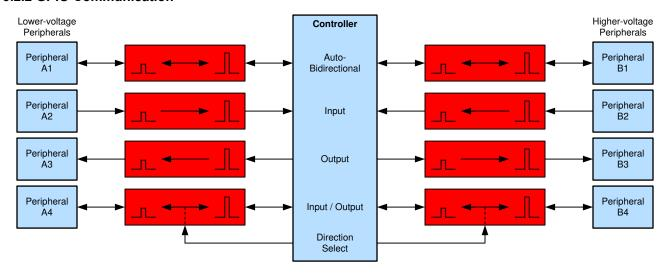
Figure 3-8. Using Voltage Translation with GPIO Communications
