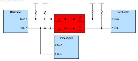
Figure 3-9. Using Voltage Translation with an I<sup>2</sup> Communication Bus
