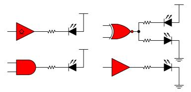
Figure 3-1. Using Logic as Indicator LED Driver Application Examples
