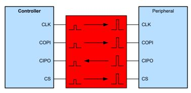
Figure 2-2. Using Voltage Translation with a SPI-Communication Bus
