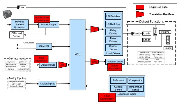
Figure 1. Simplified Body Control Module Block Diagram
