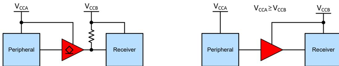
Left: block diagram for open-drain buffer. Right: block diagram for push-pull buffer.
