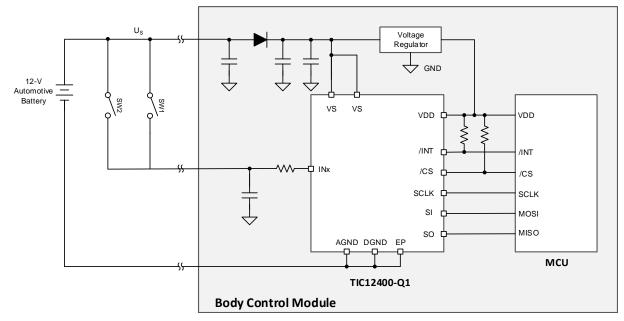
Figure 1. Typical switch detection
