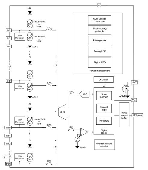
Figure 2. Simplified block diagram
