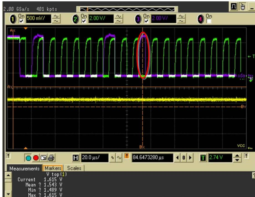
**Figure 5-1. SDA Handoff Delayed Pulldown After Ninth Clock Pulse**
