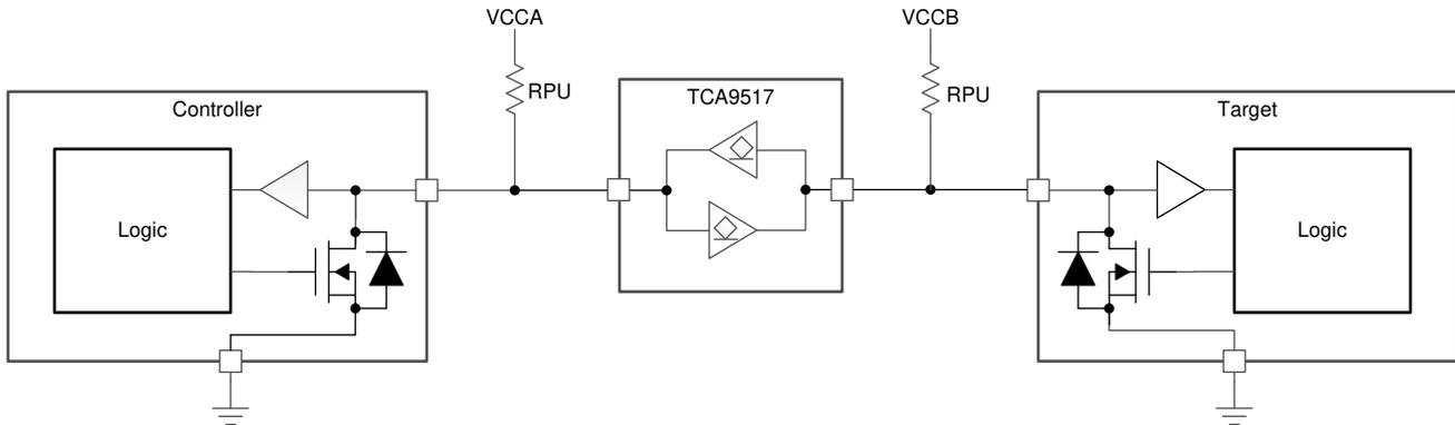
Figure 3-4. Example Setup
