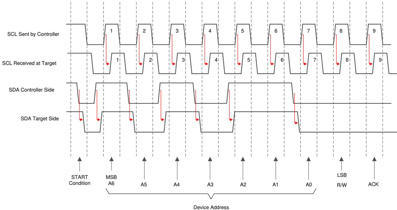
**Figure 3-1. I<sup>2</sup>C Timing With Propagation Delays From I<sup>2</sup>C Buffer**
