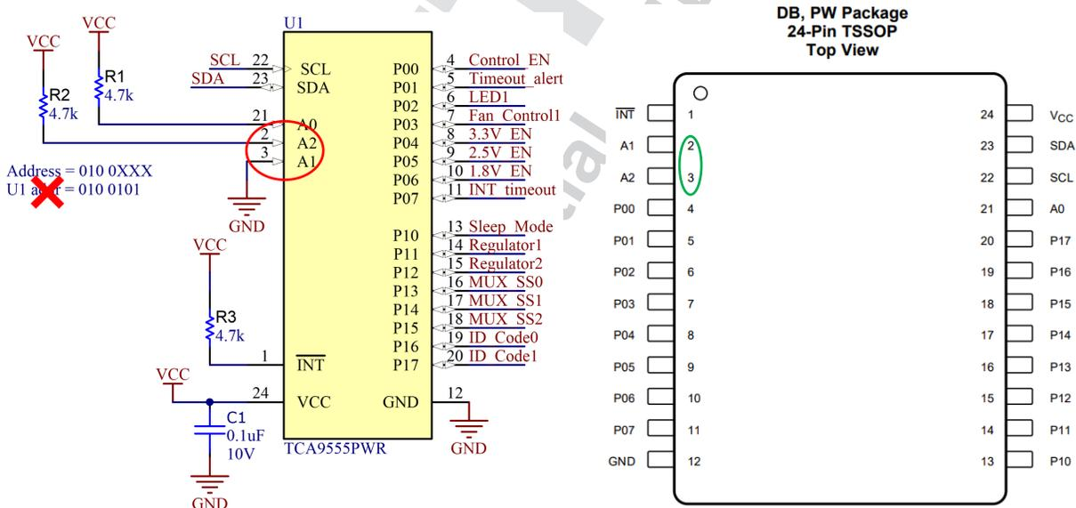
Figure 2-3. TCA9555 With Error in Schematic Revealed
