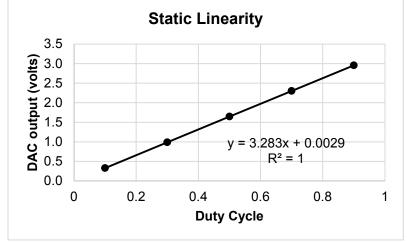
Figure 5. Example measurement data showing DAC linearity.
