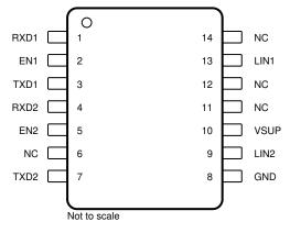
Figure 4-2. D Pin Diagram
