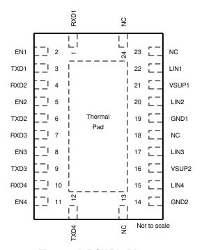
Figure 4-1. RGY Pin Diagram
