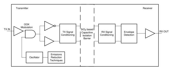
Figure 1-1. Functional Block Diagram
