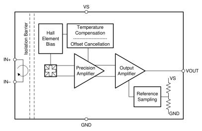
Figure 1-1. TMCS1108-Q1 Functional Block Diagram
