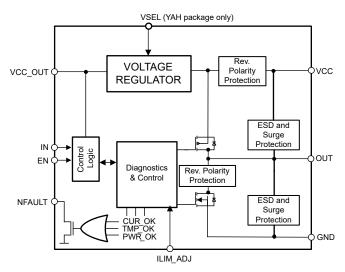
Figure 1-2. Functional Block Diagram (TIOS1023, TIOS1025)
