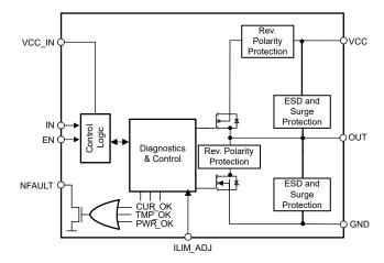
Figure 1-1. Functional Block Diagram (TIOS102)
