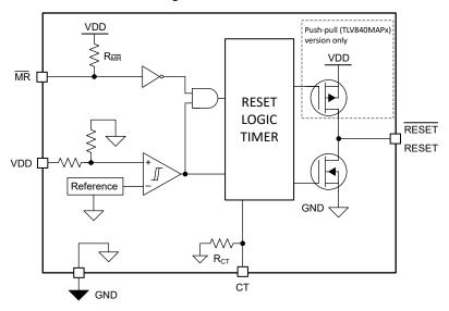
Figure 1-1. Functional Block Diagram
