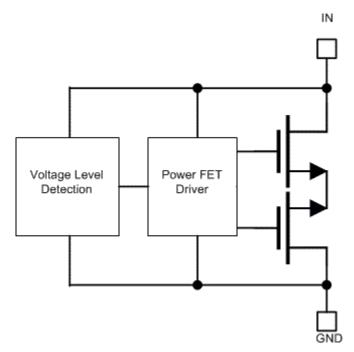
Figure 1-1. Functional Block Diagram
