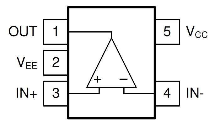
Figure 4-1. Pin Diagram (DCK and DBV) Packages
