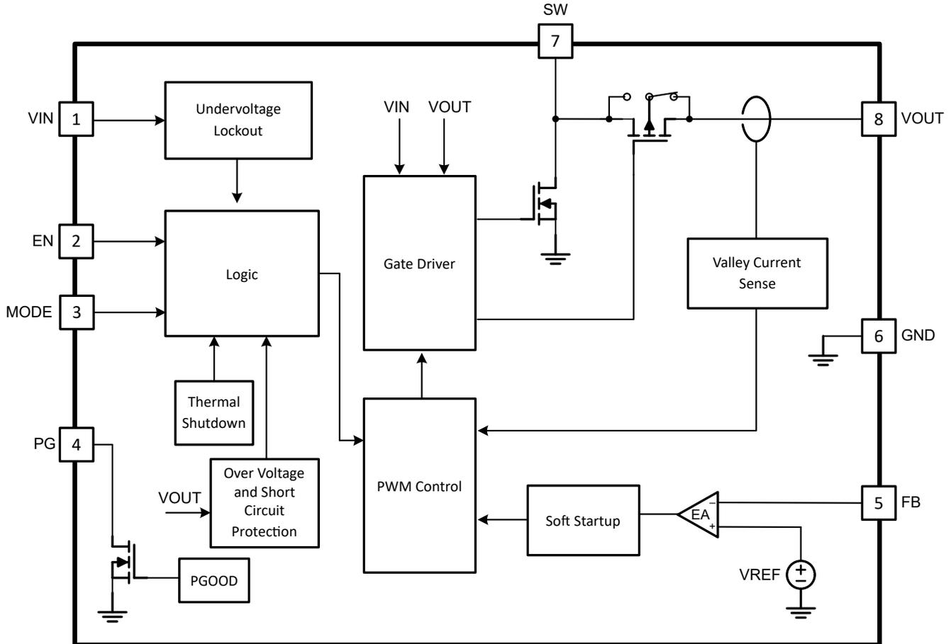
**Figure 1-1. TPS61033-Q1 & TPS610333-Q1 Functional Block Diagram**
