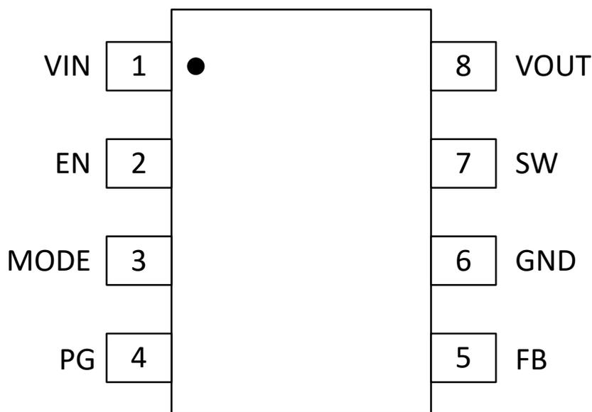
**Figure 4-1. TPS61033-Q1 and TPS610333-Q1 Pin Diagram**
