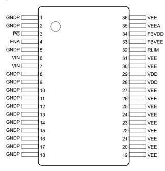
Figure 4-1. Pin Diagram (DWN-36) Package
