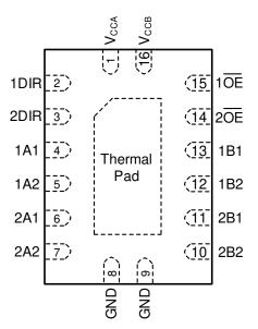
Figure 4-2. Pin Diagram (WQFN Package)
