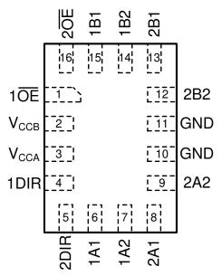
Figure 4-3. Pin Diagram (UQFN) Package
