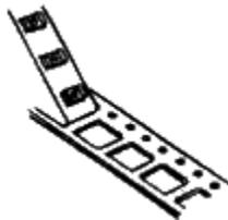
With no cover tape, components can be inspected and tested after being inserted in Surftape®.
