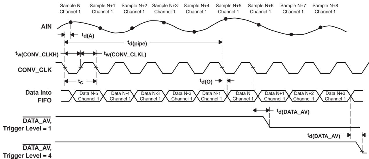
**Figure 12. Timing of Continuous-Conversion Mode (One-Channel Operation)**
