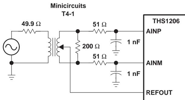
Figure 20. Single-Ended to Differential Conversion by Transformer
