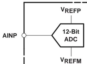
Figure 16. Single-Ended Input Stage
