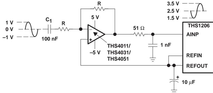
Figure 19. AC-Coupled Input
