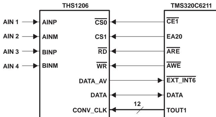
Figure 29. Interfacing the THS1206 to the TMS320C6211
