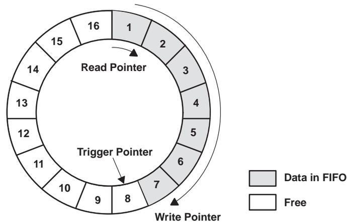
**Figure 3. The FIFO as a Circular Buffer**
