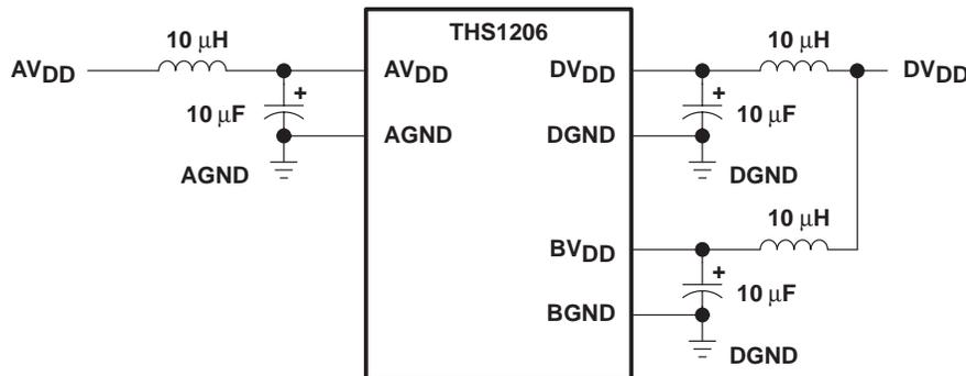
**Figure 24. Use of Bypassing With The THS1206**
