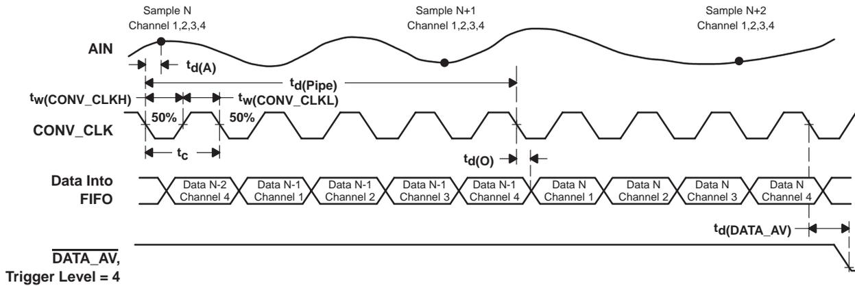
**Figure 13. Timing of Continuous-Conversion Mode (Four-Channel Operation)**
