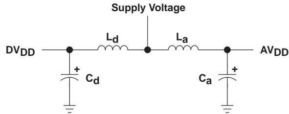
**Figure 23. Common Supply for a Mixed Signal Design**
