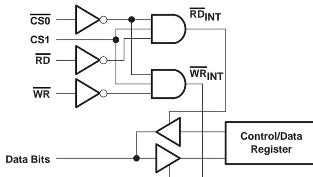
Figure 25. Logical Combination of  $\overline{CS0}$ ,  $CS1$ ,  $\overline{RD}$ , and  $\overline{WR}$
