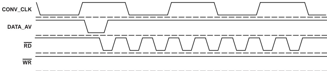
**Figure 10. Timing of DATA\_AV in Pulse Mode With Early Read**
