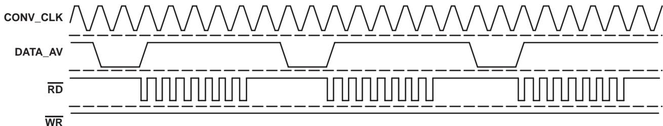
**Figure 11. Timing of DATA\_AV in Static Mode**
