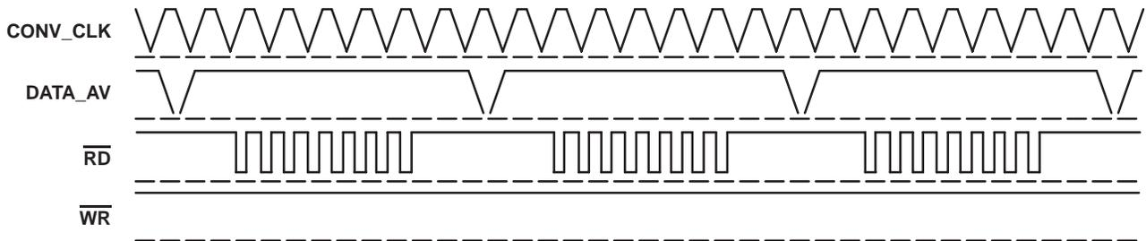
**Figure 9. Timing of DATA\_AV in Pulse Mode**
