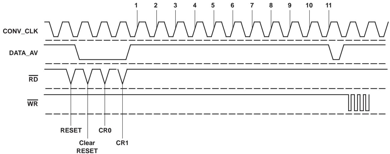
**Figure 8. DATA\_AV (In Active-Low, Pulse Configuration) After Reset**
