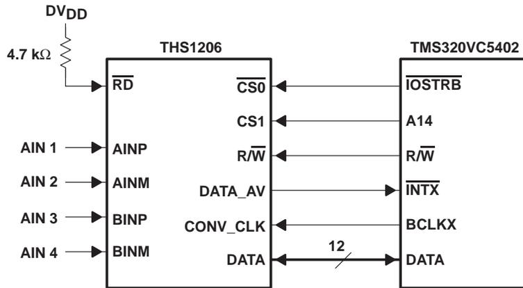
**Figure 26. Interfacing the THS1206 to the TMS320VC5402**
