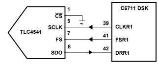
Figure 1. Hardware Interface Block Diagram
