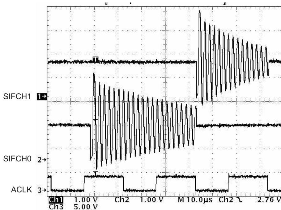
**Figure 16. Two Test Channels: Asynchronous Scan IF Timing**
