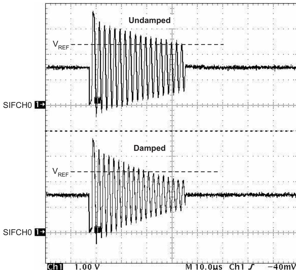
Figure 12. Undamped vs Damped Sensor Output Signals
