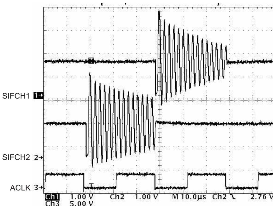
Figure 17. Two Test Channels: Synchronous Scan IF Timing
