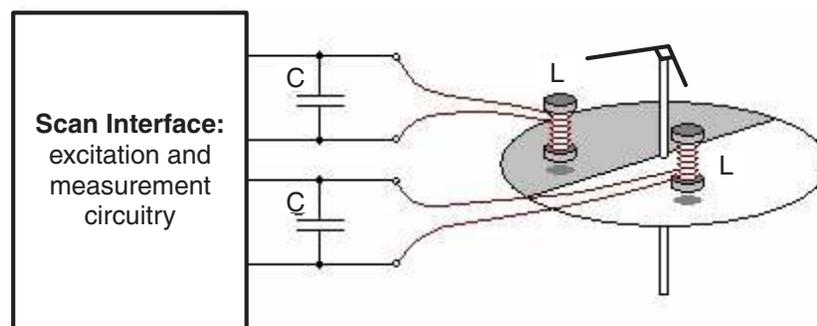
**Figure 1. Rotation Detection Using Two LC Sensors**
