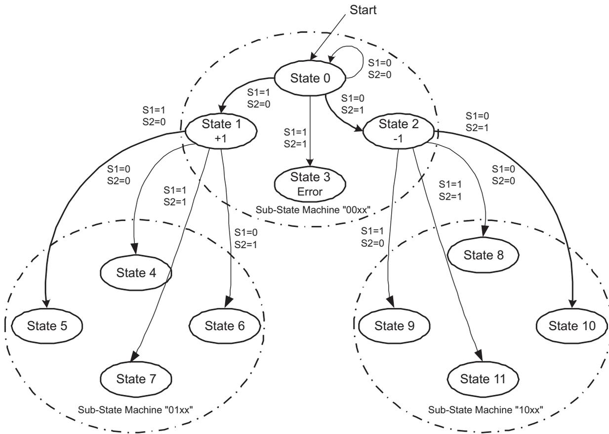
Figure 19. Two-Sensor Transition Detail
