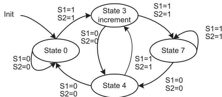
**Figure 14. Processing State Machine Example: One Sensor**
