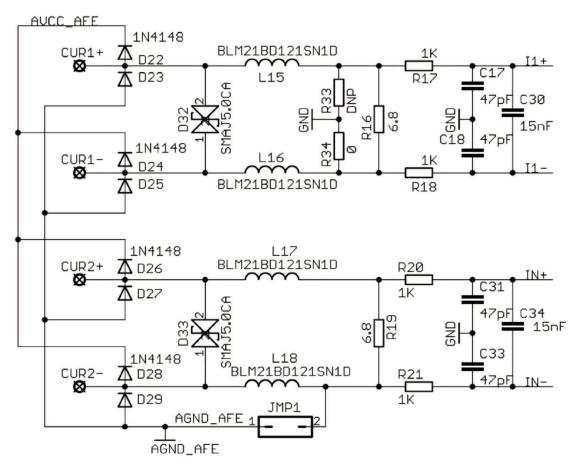
Figure 2. Analog Front End for Current Inputs
