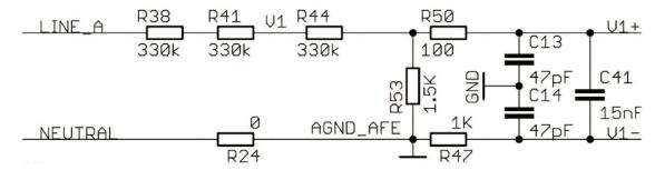
Figure 1. Analog Front End for Voltage Inputs
