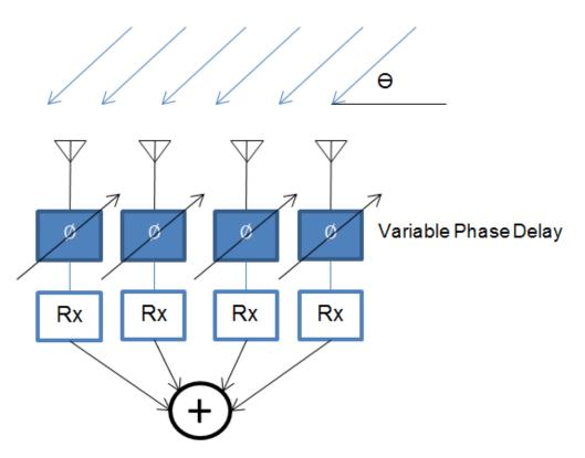
Figure 1. Phase-Array Radar Receiver System
