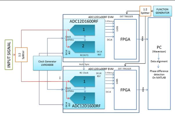
Figure 4. Multiple ADC Synchronization Test Setup
