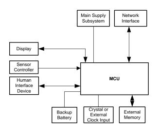
Figure 2. Example Embedded System
