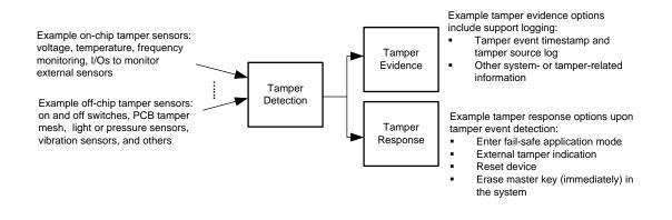
Figure 5. Tamper Protection Flow
