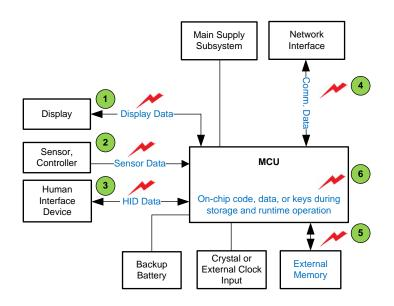
Figure 3. Typical Assets in Example Embedded System
