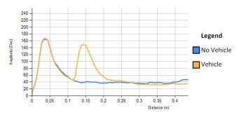
Figure 3. Occupancy Detection Below Vehicle
