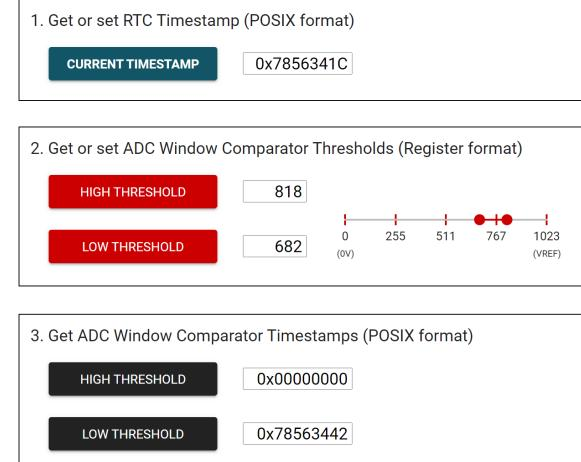
**Figure 3. Voltage Monitor with a Timestamp GUI Demo**
