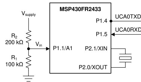
**Figure 1. Voltage Monitor Block Diagram**
