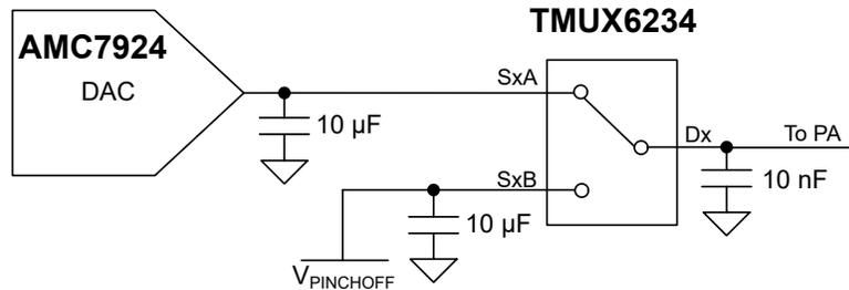
Figure 3-2. Recommended Output Switching Capacitors
