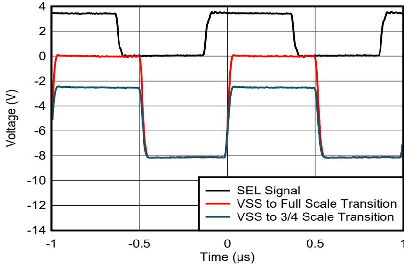
Figure 3-1. TMUX6234 Output Switching Plot
