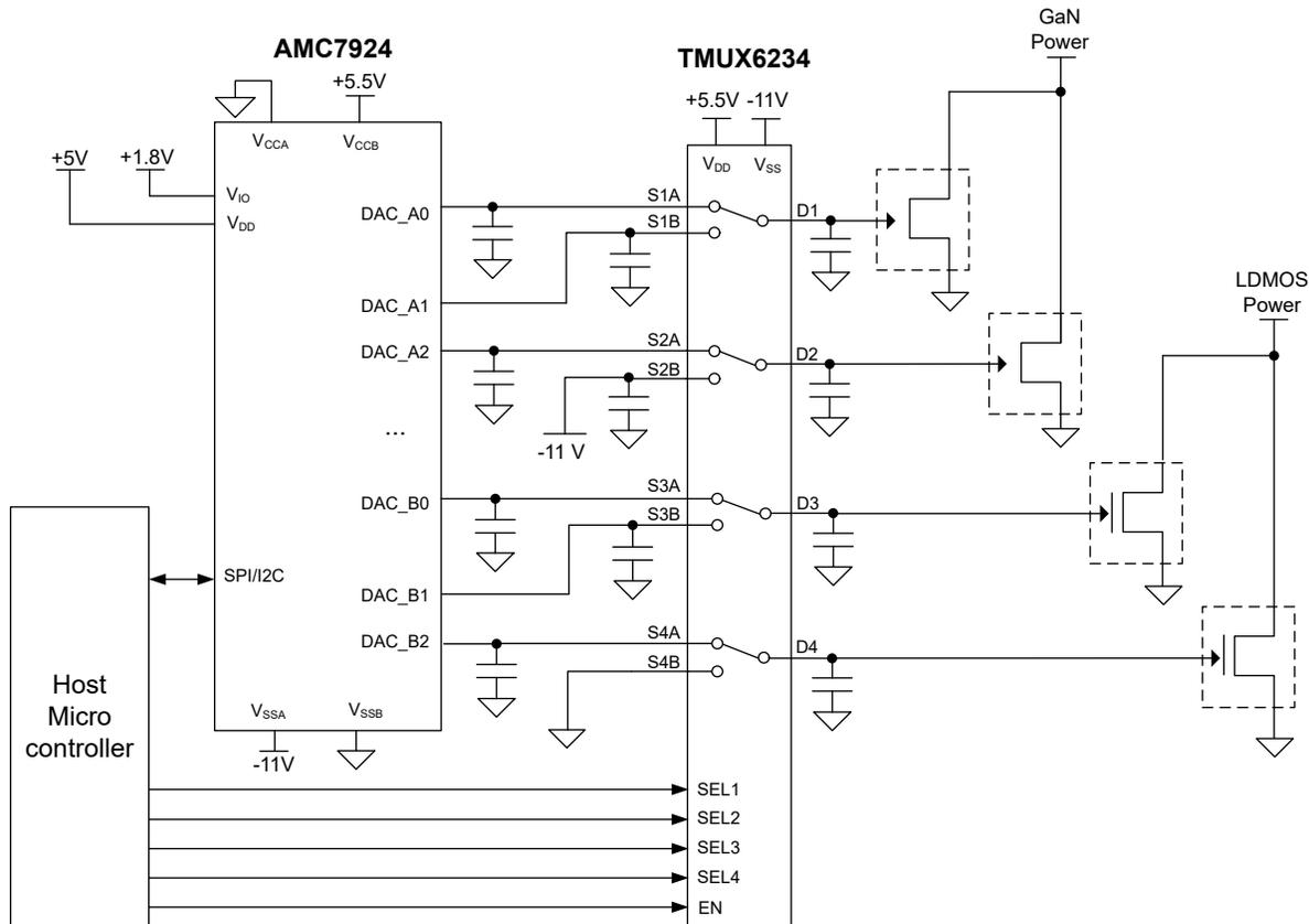
Figure 2-1. AMC7924 and TMUX6234 Application
