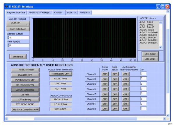
Figure 2. TI ADC SPC Interface Screen
